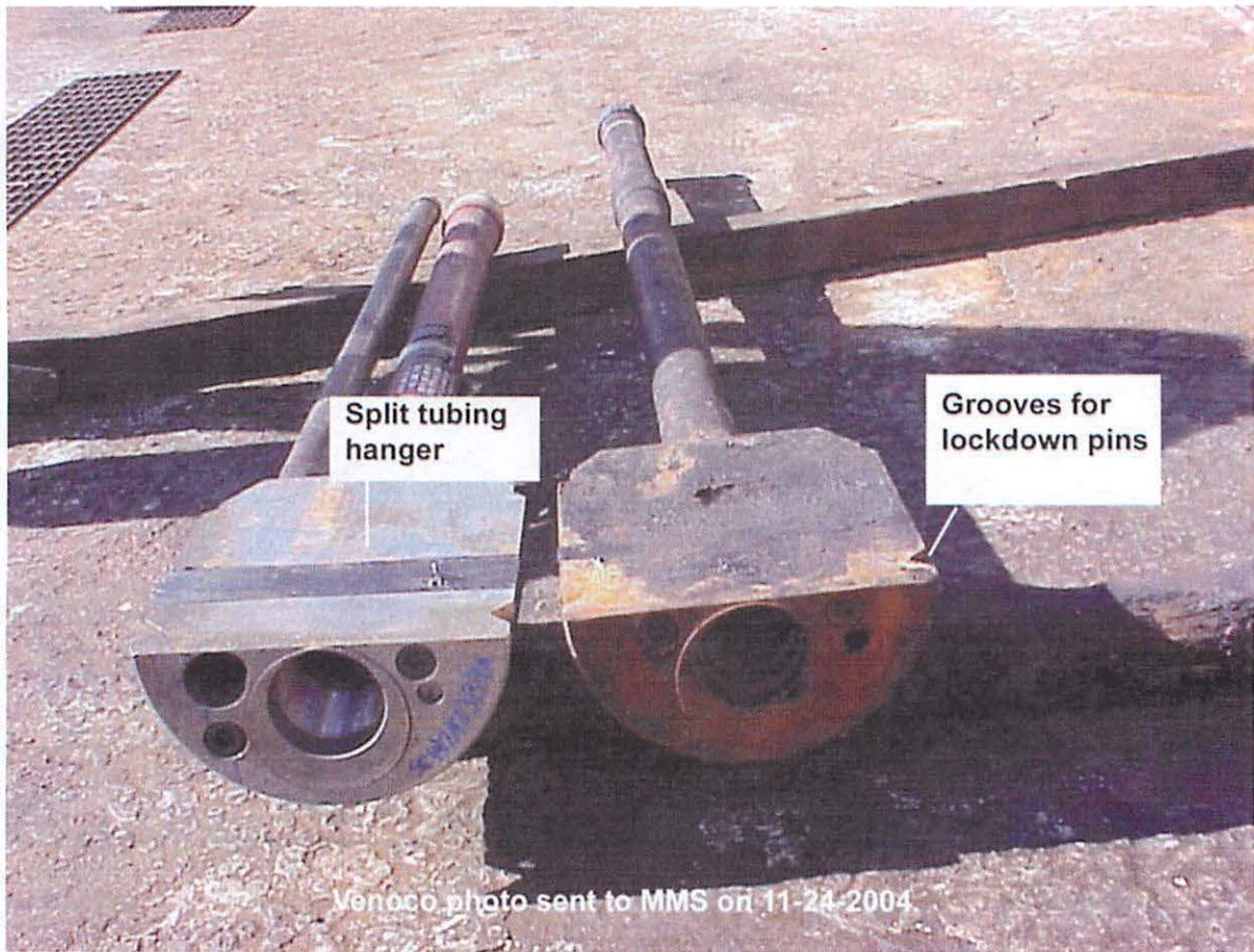
Photo showing split tubing hanger and grooves for lockdown pins on offshore oil platform.
