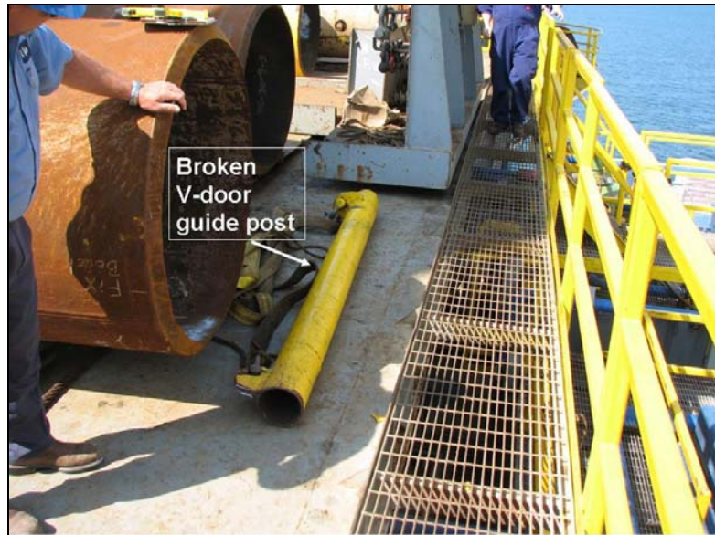
Figure 7: Broken right side V-door guide post
