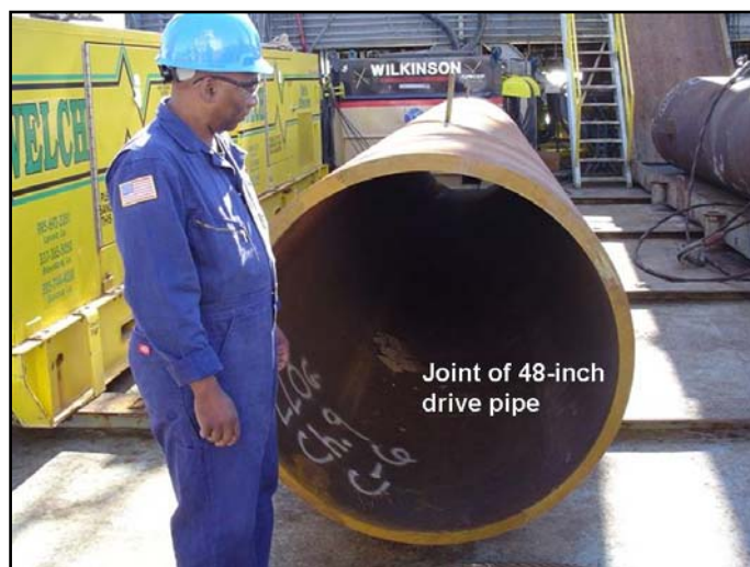
Figure 5: Example, 48-in drive pipe
