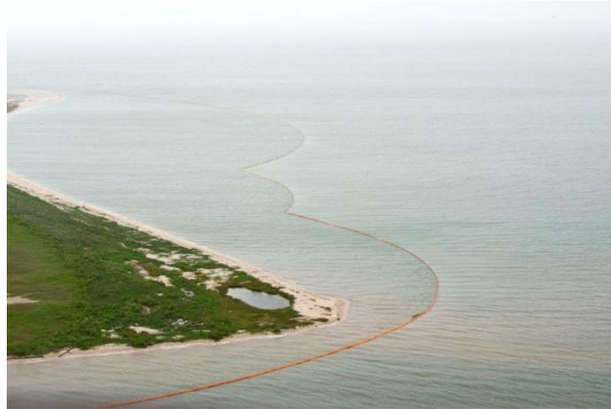
Figure 15. An example of a nearshore boom deployed (Source: USCG).
