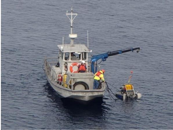
*Figure 4. Free floating brush skimmer deployed from side of vessel (Source: BSEE).*
