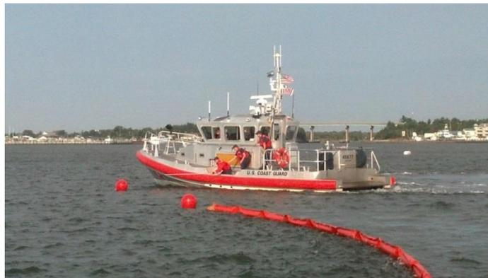
Figure 16. A nearshore deployed boom being recovered (Source: USCG).
