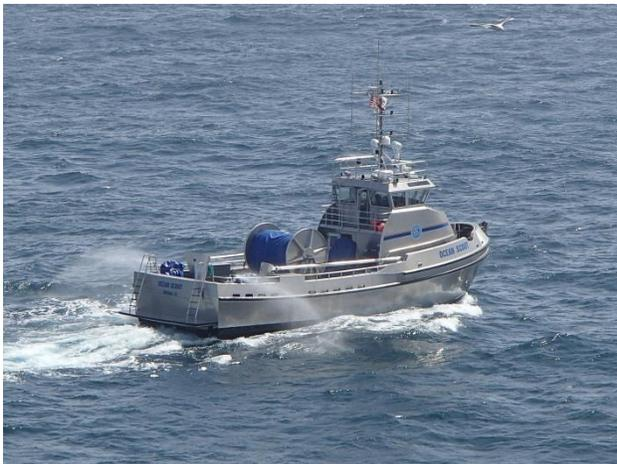
*Figure 6. A 65-ft OSRV spraying water from dispersant application system to simulate surface dispersant operations (Source: BSEE).*
