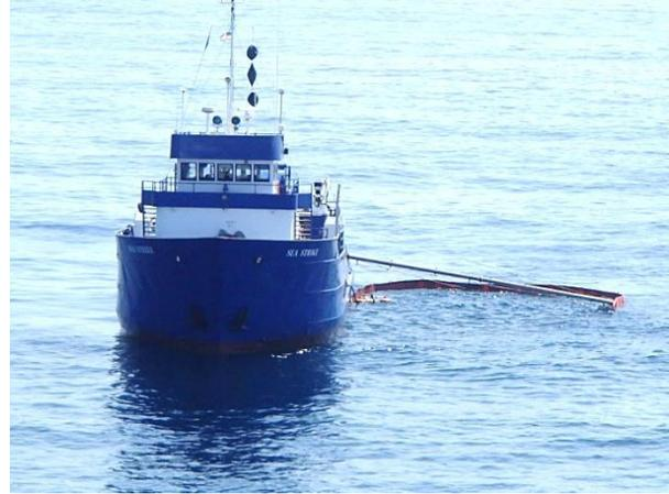
*Figure 5. Vessel deploying a side collecting boom and weir skimmer (Source: BSEE).*
