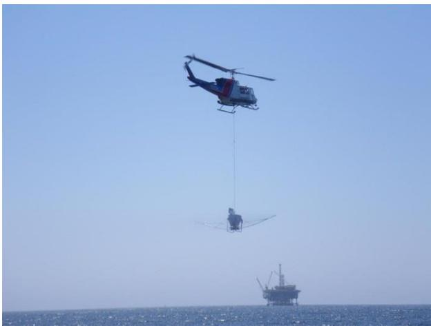
*Figure 8.* Helicopter exercising simulated dispersant application with bucket sprayer (Source: BSEE).
