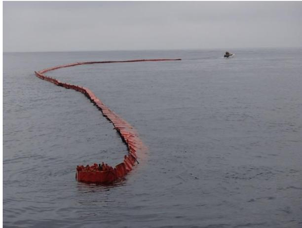
*Figure 1.* Small boat deploying curtain boom offshore (Source: BSEE).
