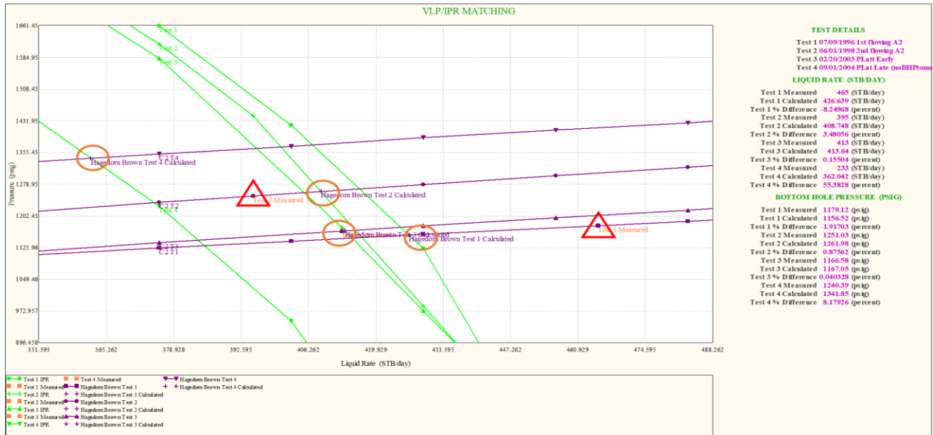
Figure 3 Zoomed in plot of simultaneous Match for all test A-02 well. Vertical axis is Pressure and Horizontal axis is liquid rate. Green Lines are the inflow performance curves and the magenta lines are the tubing performance curves. The Match point for Test 4 (Late Test – 2004) is out of the plot to the left
