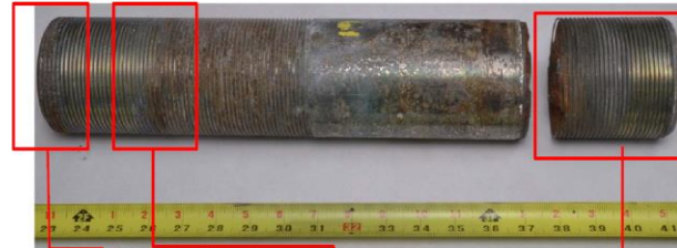
(B) After ultrasonic cleaning in an Alconox® solution. Major scale divisions are in inches.
