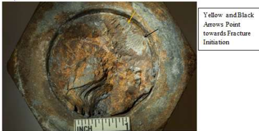
FIGURE 4: FRACTURE INITIATION AT NUT END (BSEE RCA)
