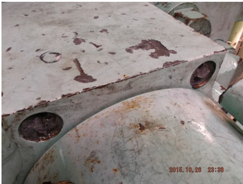
FIGURE 6: UPPER BSR FASTENER FAILURES – CLOSE-UP OF SHEARED THREADS
