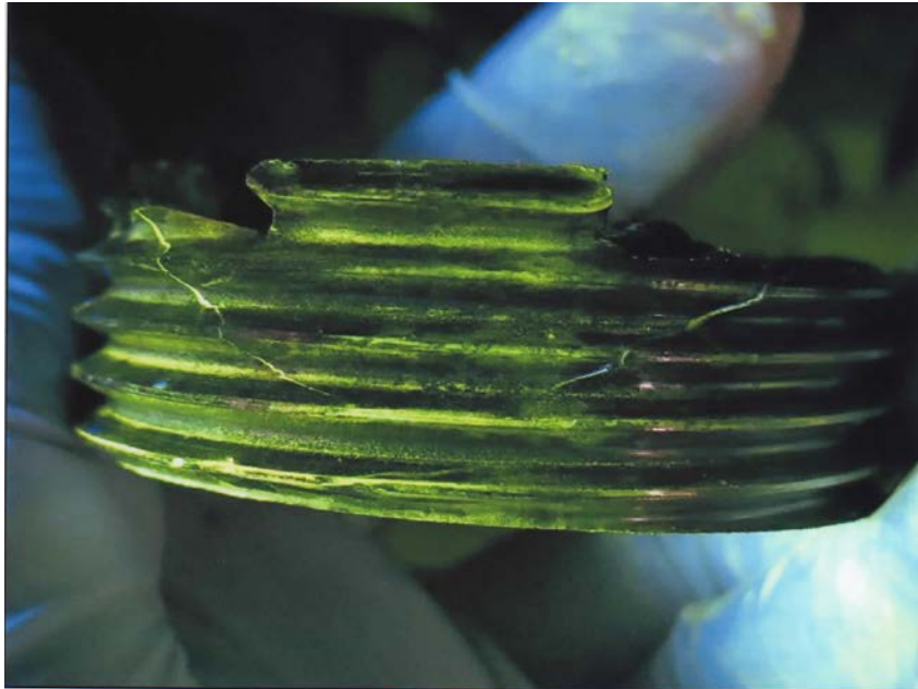
FIGURE 9: CRACK PROPAGATION THAT EXTEND INTO MULTIPLE THREADS BELOW THE FRACTURE FACE (OEM RCA)
