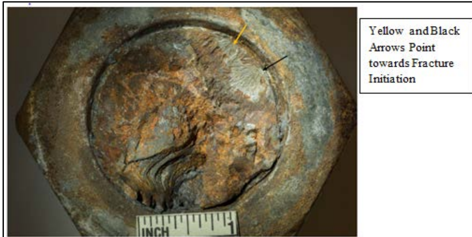
FIGURE 13: FRACTURE INITIATION AT NUT END (NASA RCA)
