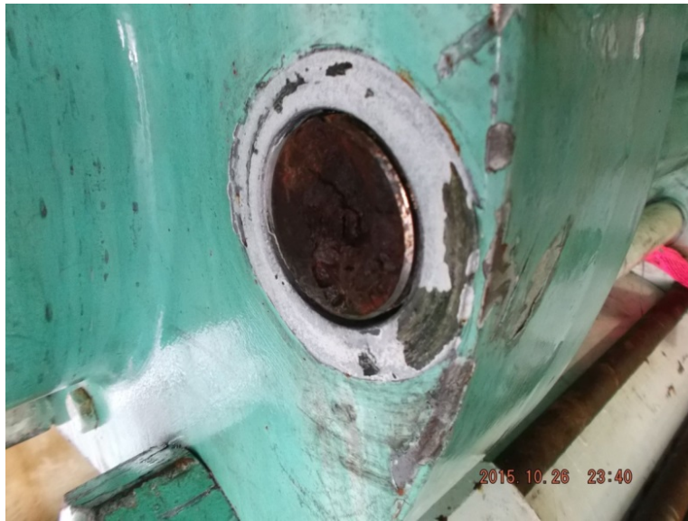
FIGURE 7: UPPER BSR FASTENER FAILURES – CLOSE-UP OF SHEARED FASTENER
