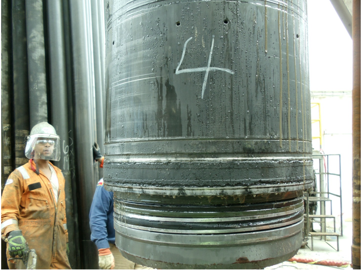
FIGURE 2: PULLED SUB MUDLINE CASING HANGER SEAL
