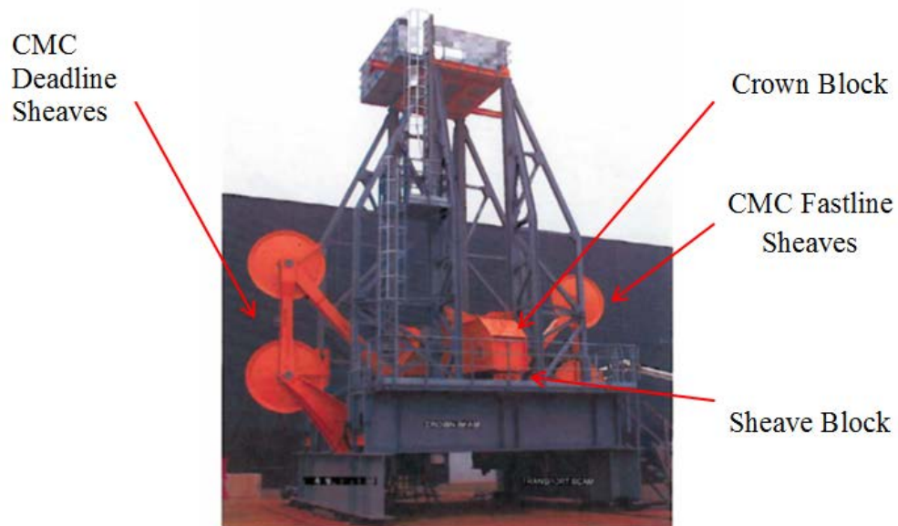
FIGURE 2: CMC ASSEMBLY - SHEAVES ARE INTERCHANGEABLE (OEM USER MANUAL)
