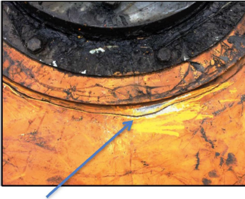
Illustrations: Above: Example of crack at hub of old fastline sheave. Right: Cross-section of typical sheave. The red arrows are pointing at the welds that supplier defines as "critical".
