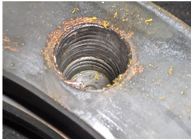
Figure 6: Stripped threads in the retainer ring and depth of thread engagement
