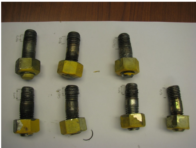
Figure 7: Failed Fasteners and stripped threads
