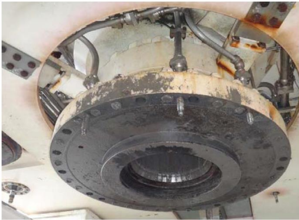
Upper half of failed LMRP Connector
