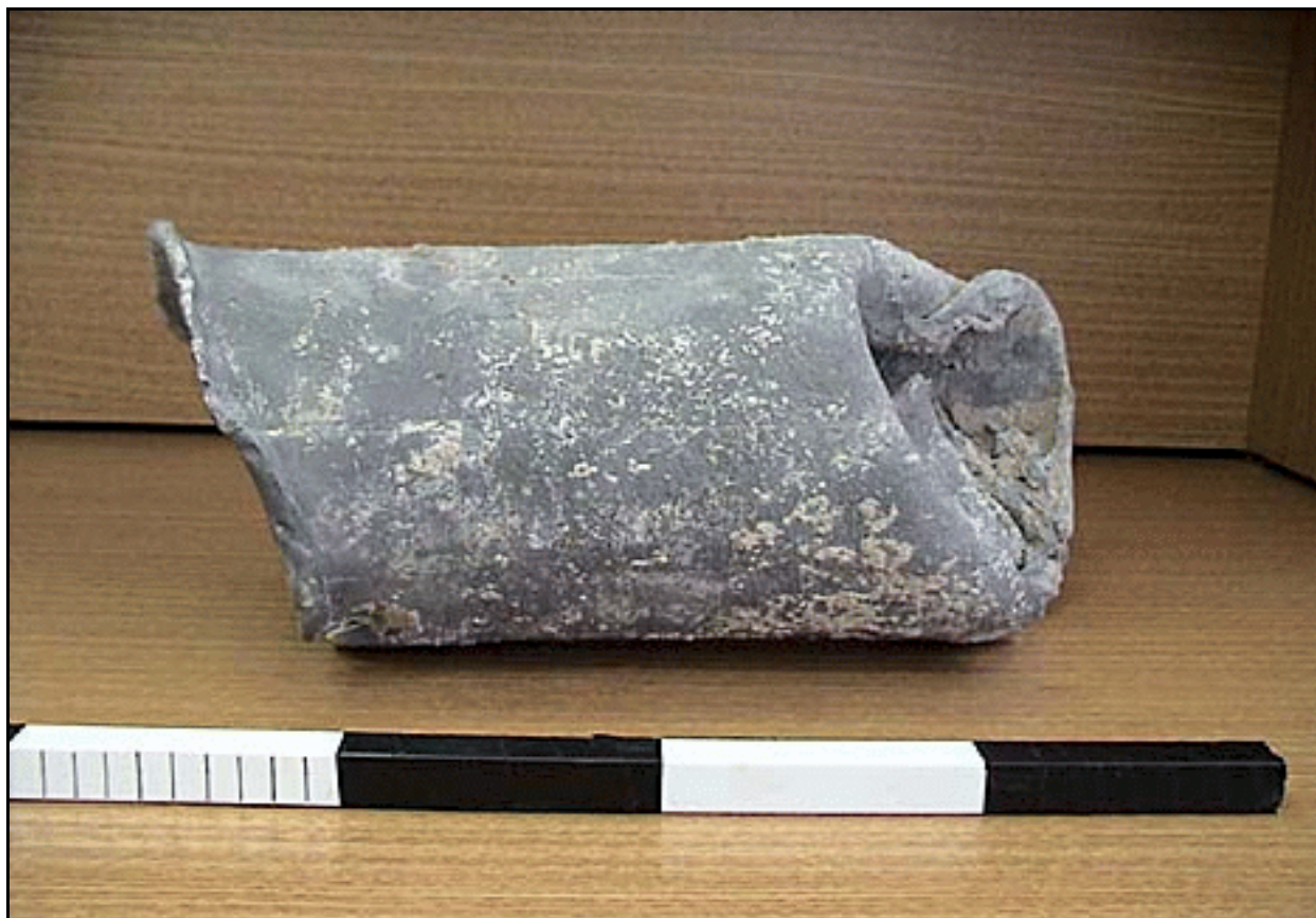
Figure 1C.3. Hawsepipe, recovered from bow of vessel.
