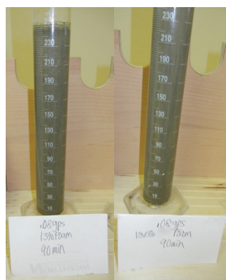
Figure #13. Pictures on the left show the 0.08 gps SCR-100 slurry that was pre-conditioned for 1.5 hours and tested for Foam Stability at 13% (l) and 18.5% (r) Foam Quality right after mixing. Pictures on the right show the 0.09 SCR-100 gps slurry that was pre-conditioned for 1.5 hours and tested for Foam Stability at 13% (l) and 18.5% (r) Foam Quality right after mixing.
