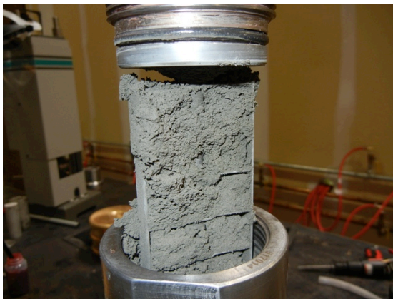
Figure #10. Fluid Loss specimen after test blew dry (0.08 gps SCR-100 system with 83 minute conditioning time).
