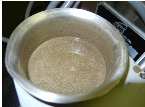
Figure #5. Compatibility between 25% base slurry and 75% drilling fluid.
