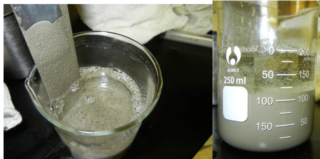
Figure #4. Compatibility between 50% base slurry and 50% base oil.
