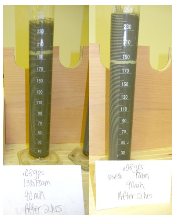
Figure #14. Pictures on the left show the 0.08 gps SCR-100 slurry that was pre-conditioned for 1.5 hours and tested for Foam Stability at 13% (l) and 18.5% (r) Foam Quality after 2-hour period. Pictures on the right show the 0.09 SCR-100 gps slurry that was pre-conditioned for 1.5 hours and tested for Foam Stability at 13% (l) and 18.5% (r) Foam Quality after 2-hour period.
