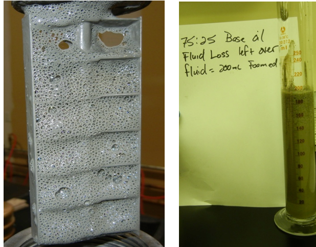
Figure #11. Fluid Loss test specimen after 30 minutes for the 75% 0.09 gps SCR-100 base slurry with 25% base oil contamination (with 83 minute conditioning time).
