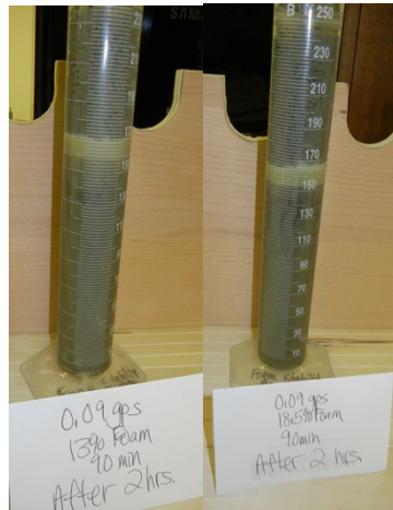
Figure #21. Pictures show 0.09 gps SCR-100 slurry testing for Foam Stability and Foam Quality after a 2-hour quiescent period, pre-conditioned for 1.5 hours (left set) and 3 hours (right set). In each pair of cylinders, the targeted 13% foam quality (15.3% true) is on the left and the targeted 18.5% (21.8% true) is on the right.
