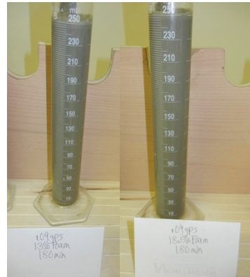
Figure #15. Pictures on the left show the 0.08 gpm SCR-100 slurry that was pre-conditioned for 3 hours and tested for Foam Stability at 13% (l) and 18.5% (r) Foam Quality right after mixing. Pictures on the right show the 0.09 SCR-100 gpm slurry that was pre-conditioned for 3 hours and tested for Foam Stability at 13% (l) and 18.5% (r) Foam Quality right after mixing.
