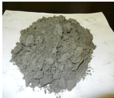
Figure #10. Fluid Loss specimen after test blew dry (0.08 gps SCR-100 system with 83 minute conditioning time).
