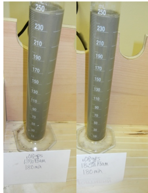
Figure #15. Pictures on the left show the 0.08 gpm SCR-100 slurry that was pre-conditioned for 3 hours and tested for Foam Stability at 13% (l) and 18.5% (r) Foam Quality right after mixing. Pictures on the right show the 0.09 SCR-100 gpm slurry that was pre-conditioned for 3 hours and tested for Foam Stability at 13% (l) and 18.5% (r) Foam Quality right after mixing.
