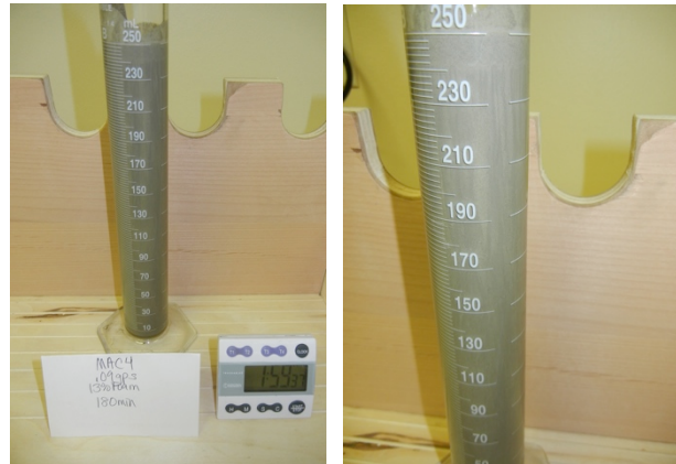
Figure #17. Pictures above show the MAC4 Macondo cement 0.09 gps SCR-100 slurry that was pre-conditioned for 3 hours and tested for Foam Stability at 13% Foam Quality right after mixing.
