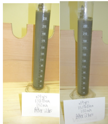
Figure #16. Pictures on the left show the 0.08 gpm SCR-100 slurry that was pre-conditioned for 3 hours and tested for Foam Stability at 13% (l) and 18.5% (r) Foam Quality after 2-hour period. Pictures on the right show the 0.09 SCR-100 gpm slurry that was pre-conditioned for 2 hours and tested for Foam Stability at 13% (l) and 18.5% (r) Foam Quality after 2-hour period.
