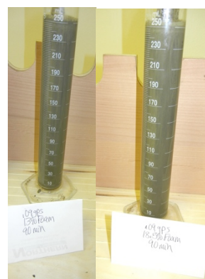
Figure #13. Pictures on the left show the 0.08 gps SCR-100 slurry that was pre-conditioned for 1.5 hours and tested for Foam Stability at 13% (l) and 18.5% (r) Foam Quality right after mixing. Pictures on the right show the 0.09 SCR-100 gps slurry that was pre-conditioned for 1.5 hours and tested for Foam Stability at 13% (l) and 18.5% (r) Foam Quality right after mixing.
