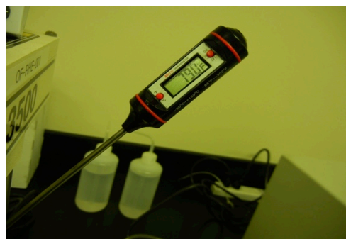
Figure #3. A heated cup was used for all rheology tests to regulate temperature and a thermometer was used to measure temperature.
