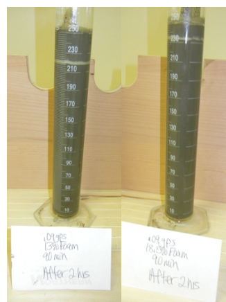
Figure #14. Pictures on the left show the 0.08 gps SCR-100 slurry that was pre-conditioned for 1.5 hours and tested for Foam Stability at 13% (l) and 18.5% (r) Foam Quality after 2-hour period. Pictures on the right show the 0.09 SCR-100 gps slurry that was pre-conditioned for 1.5 hours and tested for Foam Stability at 13% (l) and 18.5% (r) Foam Quality after 2-hour period.
