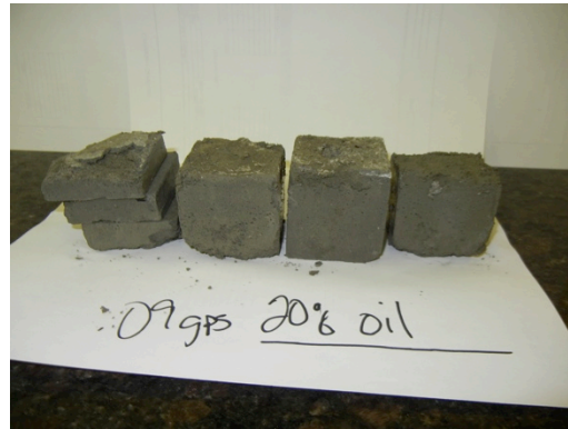
Figure #19. Picture above shows the 0.09 gps SCR-100 slurry with 20% base oil contamination that was pre-conditioned for 3 hours and tested for Foam Stability at 13% Foam Quality. Cement cubes were not hard set after 48 hour curing period.
