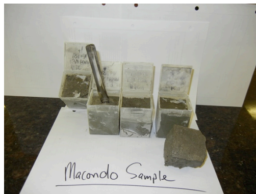
Figure #20. Picture above shows the MAC4 Macondo cement 0.09 gps SCR-100 slurry that was pre-conditioned for 3 hours and tested for Foam Stability at 13% Foam Quality. Cement cubes were not hard set after 48 hour curing period.
