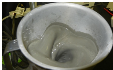
Figure #2. Base slurry was mixable and a clear vortex was visible.
