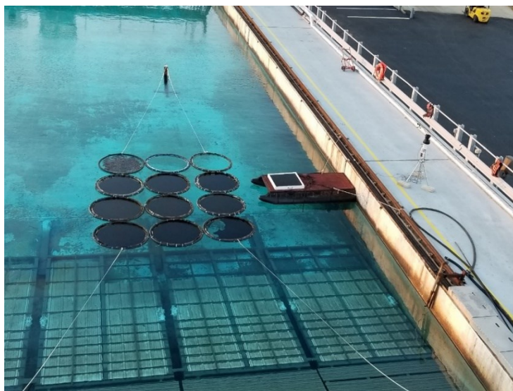
Figure 2. Photograph of the experimental set-up at Ohmsett, showing crude oils contained in 1.5 m diameter rings, blackbody calibration source, and weather station.
