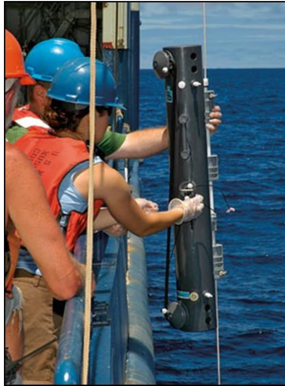
Figure C-18. Larger size GO-FLO sample bottle rigged for deployment.
