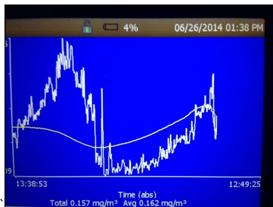
Figure C-6. TSI DustTrak DRX 8533 air monitor touch screen showing a graphical view of instantaneous and TWA particle concentration values.
