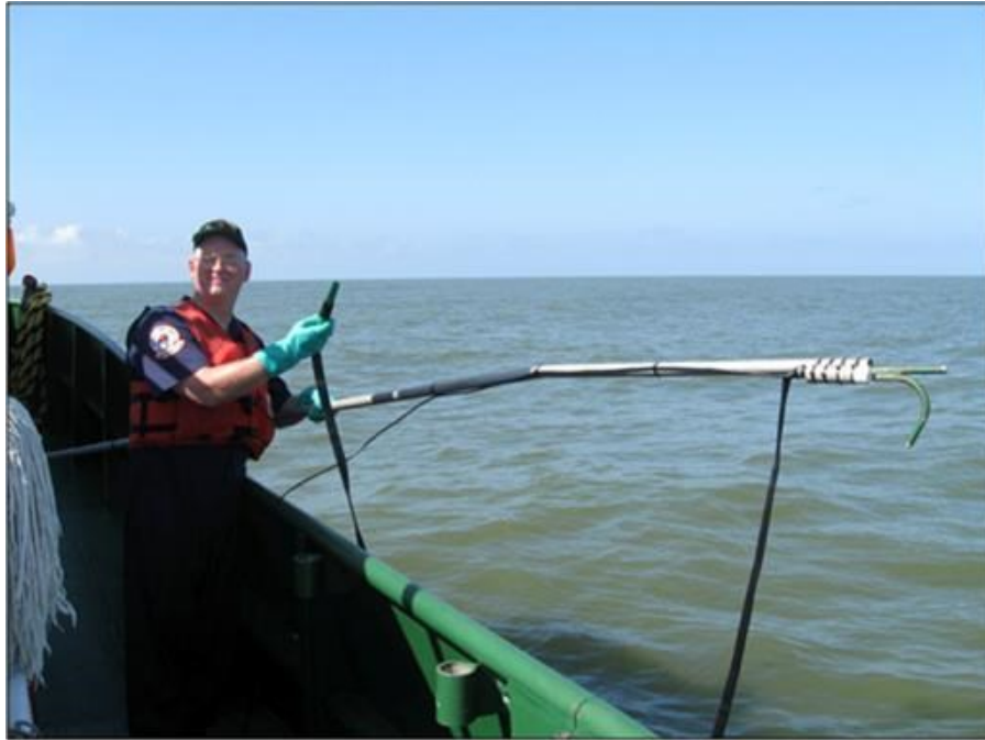
Figure A-5. Improvised water sampling pump for 5 m samples.
