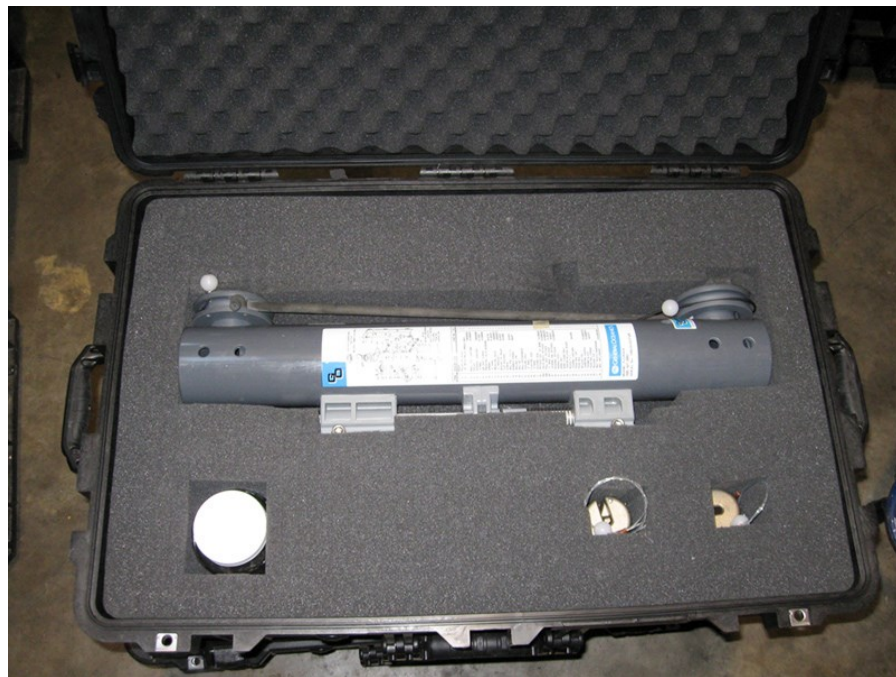
Figure A-6. GO-FLO water sample bottle for 10 m samples.
