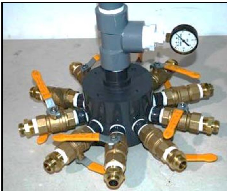
Figure 15. Circular manifold for air distribution to the ten bubble generators.
