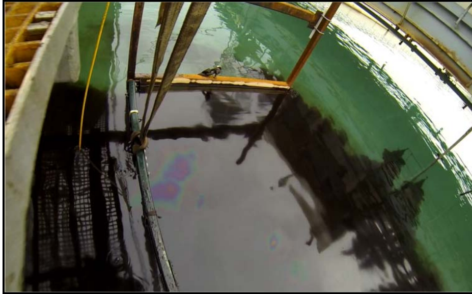
Figure 9. Example of oil plume being “pushed” by frame.
