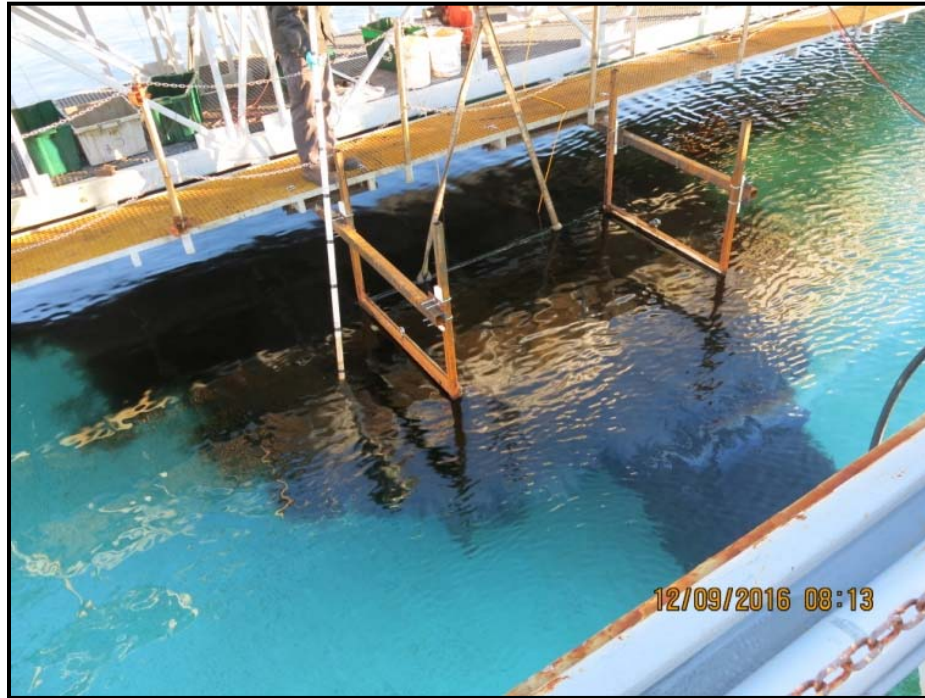
Figure 8. Example of oil plume around and behind the frame.
