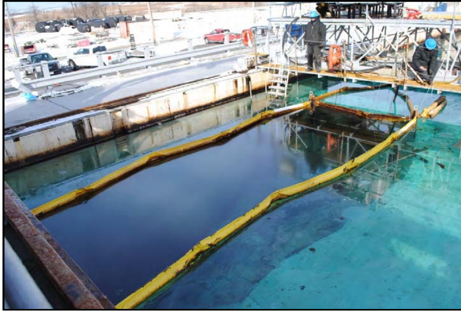
Figure 17. Isolated test section in the Ohmsett tank.
