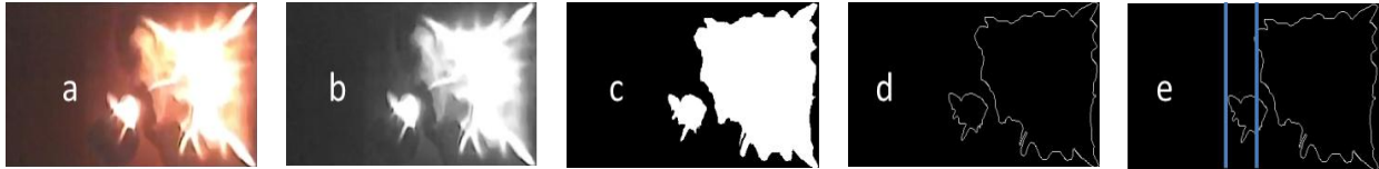
Fig. 5.3: (a) real flame (b) binary flame (c) binary filled flame (d) flame edge (e) flame length measurement range.
