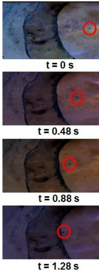
Fig. 3.7: Movement of a soot particle on the surface of the fuel. The particle traveled a length of 1.5 cm in 1.28 seconds towards the ice wall. Solid ice, ice cavity, and fuel surface from left to right.
