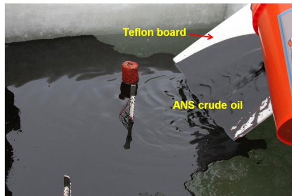
Fig. 6.6: Pouring of ANS crude oil in an ice cavity using a Teflon board to prevent spillage.
