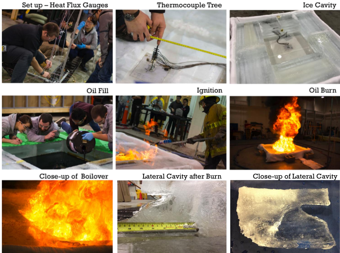
Fig. 6.3: Photographic record of large scale indoor test using Alaska North Slope (ANS) crude oil
