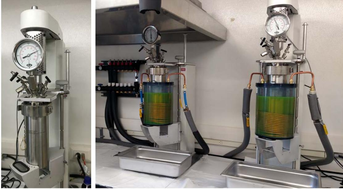
**Figure 4.1.** Examples of a non-mixing (left) and mixing reactor (right) fitted with the ethylene glycol cooling systems (with insulation removed to show the cooling coils. The wall-mounted manifold to the left allows for independent control of cooling to each of the six reactors. The image on the right shows a mixing reactor without the cooling system.
