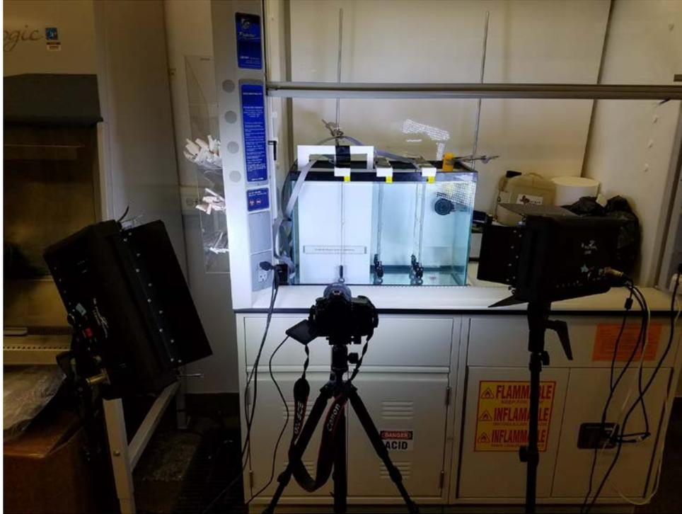
**Figure 4.33.** Laboratory setup for the blowout tank.
