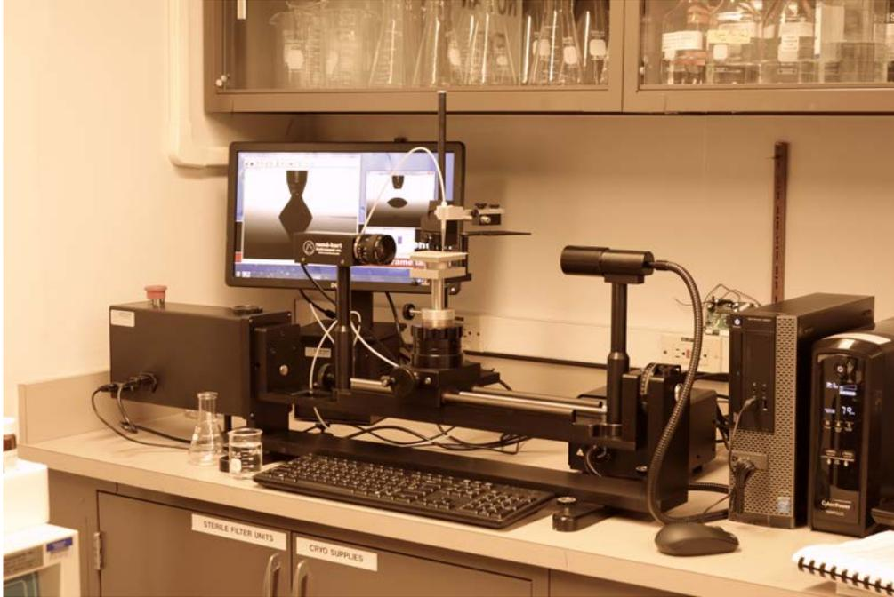
**Figure 4.3.** A ramé-hart 590-U1 Advanced Automated Goniometer/Tensiometer used to measure contact angle of oil on surfaces to determine the oleophobicity of a surface and to measure the interfacial tension between fluids.
