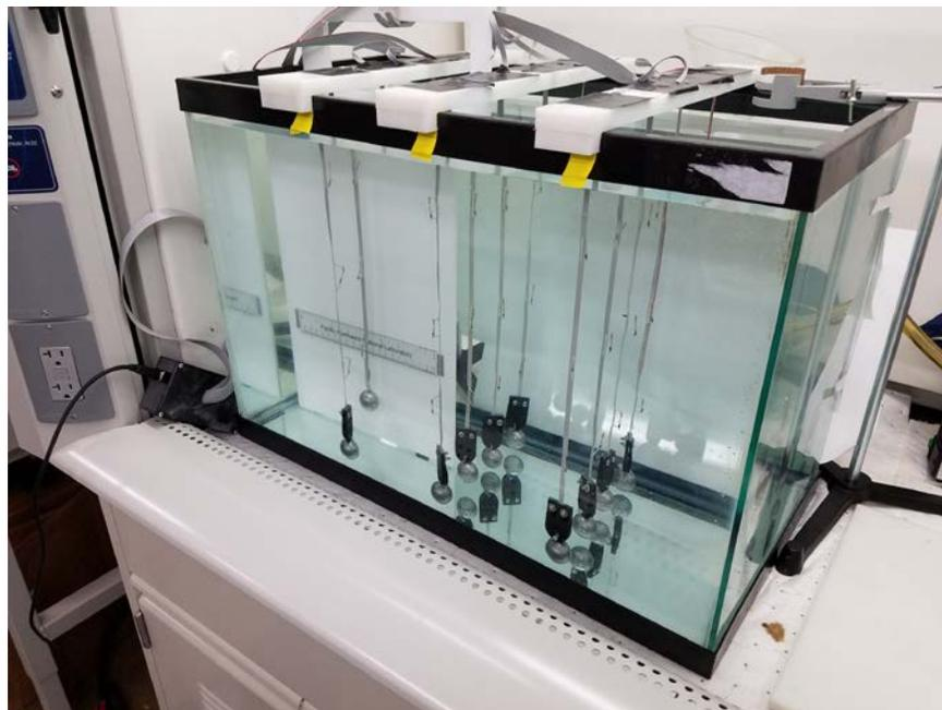
**Figure 4.32.** Test tank showing a 4×3 thermal probe array. Each wire had three thermistors along its length to interrogate the top, middle, and bottom depths of the tank.
