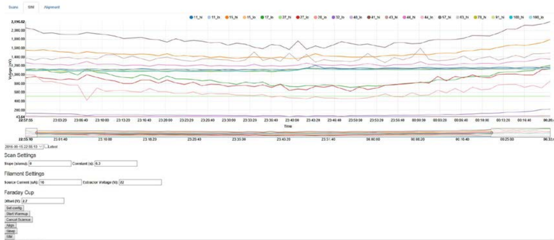
Figure 6: Screen capture of web-based mass spectrometer controller and data visualizer, showing SIM data collected during glider dive operations and transmitted over radio link while the vehicle was surfaced.
