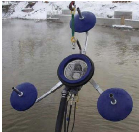
Fig. 84-Lamor LWS-50 Wier Skimmer. Photographed just before use. [65]
