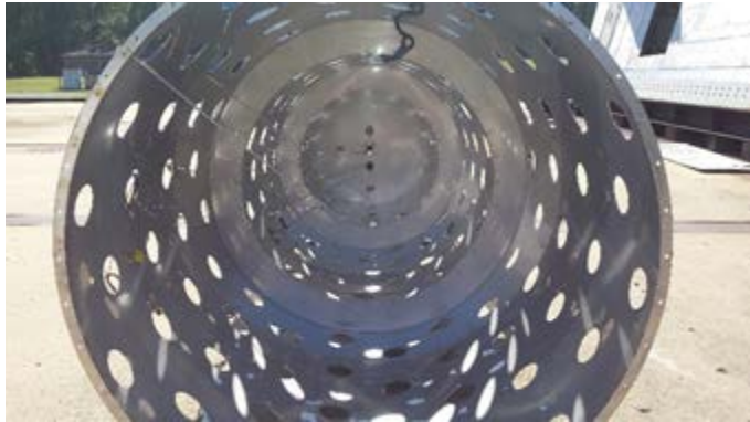
Fig. 12-Photograph of the inside of the instrumented combustor shroud.
