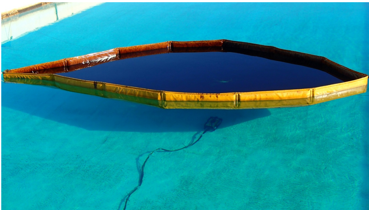
Figure 3. The arbitrary shaped boom configuration tested at Ohmsett more closely simulated an operational environment by allowing for more maneuverability under the slick, less control over the surface area and slick thickness.
