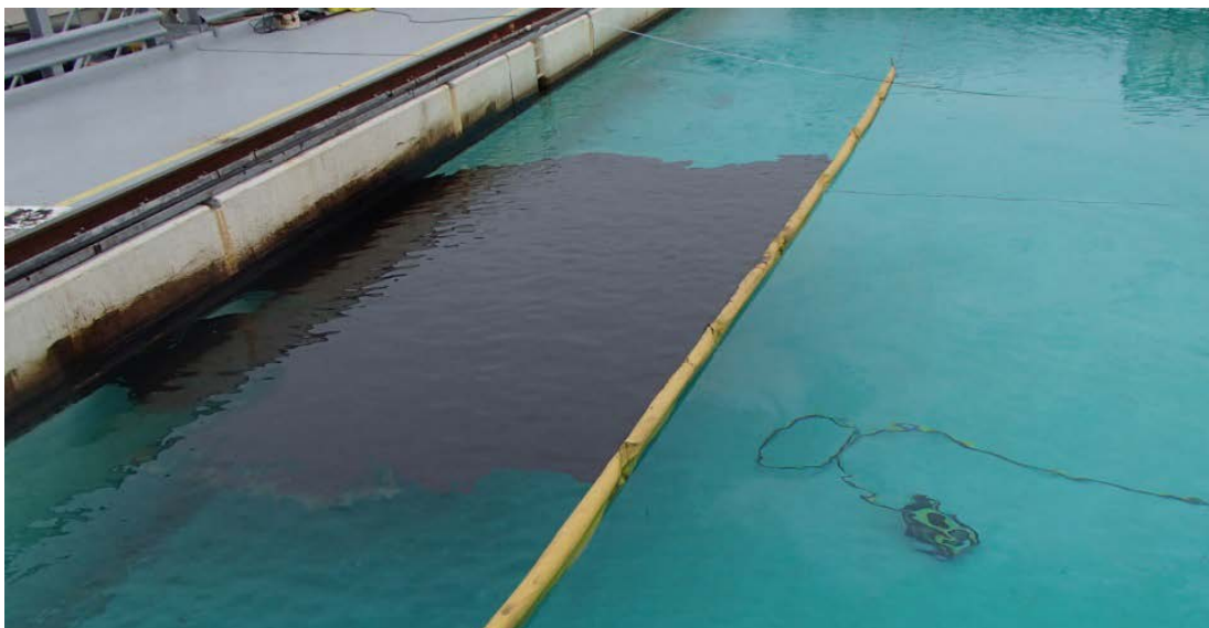
Figure 2. A linear boomed area was filled with 70 L to 132 L of ANS oil and contained with ice eaters at either end to prevent oil loss during testing.
