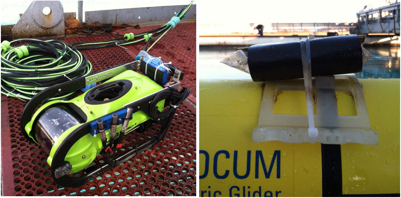
Figure 2: Mounting of the measurement device. Showing position of measurement device on (a) Seabotix ROV and (b) Slocum Glider. Waterproof case was placed inside of a protective pressure-resistant bag with air removed to protect from crude oil contamination.
