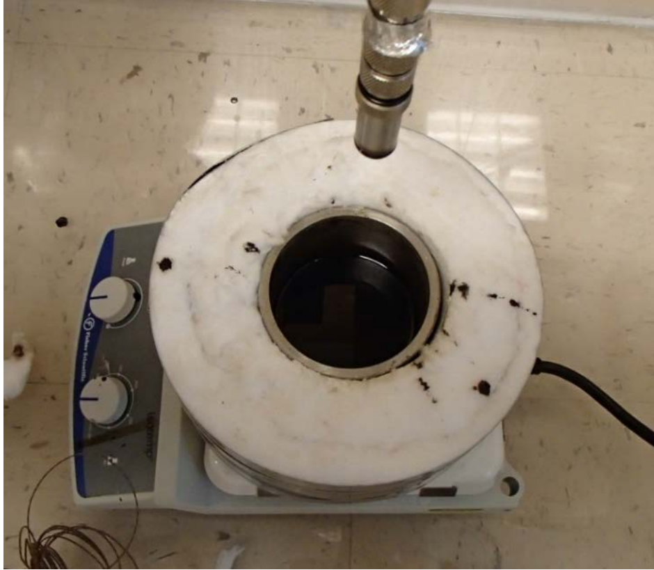
Figure 15. The cylindrical oil container was wrapped with insulation fiber to maintain temperature.
