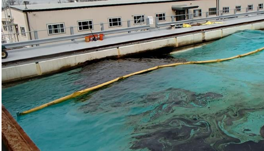
Figure 7. Waves varied in height throughout the experiments at Ohmsett; the waves made during Test 17 had a mean height of 21.4 Inches and wavelength of 39.3 Feet.
