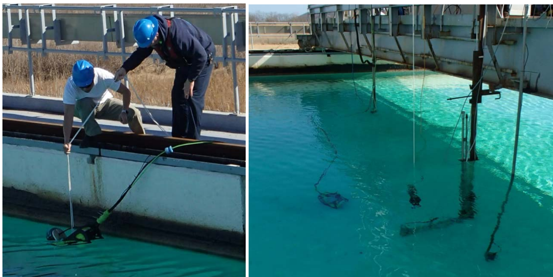
Figure 41. The ROV was deployed in the tank by carefully lowering over the side (Left) before maneuvering near the bubble generator (Right).
