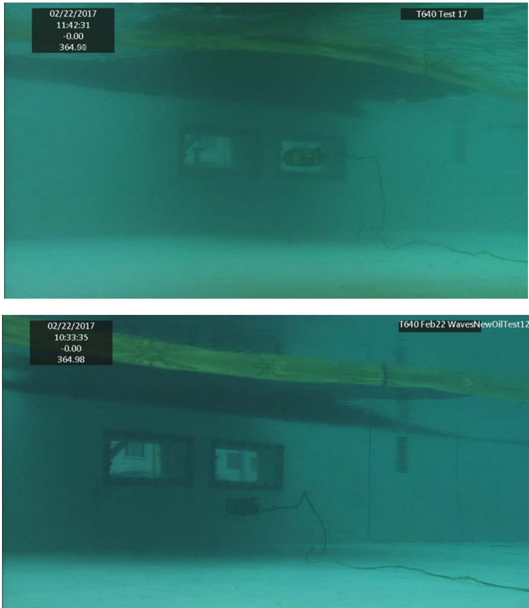
Figure 19. The ROV performed acoustic measurements of oil slick thickness at two depths – 1.2 meters (top) and 1.8 meters (bottom).
