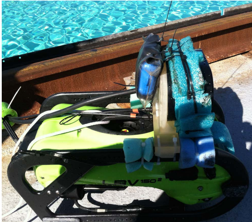
Figure 17: Mounting of the measurement device on the ROV during subsurface release testing. Note that measurement device is mounted directly posterior to the low-frequency transducer (shown wrapped with buoyancy foam).
