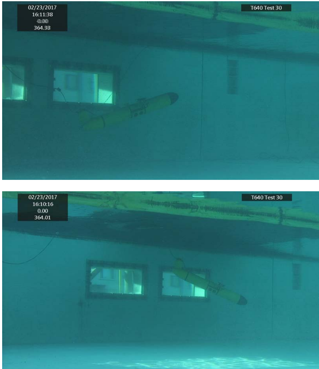
Figure 34. The glider was programmed to perform a standard yo profile ( \pm 26 degrees) spanning the 8 foot depth of the water column.
