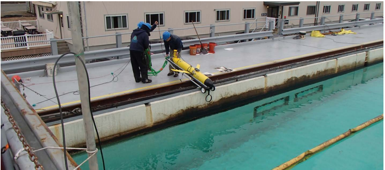
Figure 32. The glider was deployed into the tank from the side using deployment techniques similar to techniques used in the open water.
