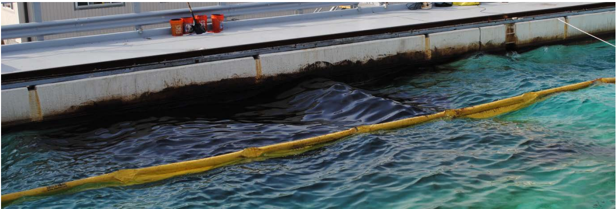
Figure 8. Waves varied in height throughout the experiments at Ohmsett; the harbor chop made during Test 20C had a mean height of 6.0 Inches and wavelength of 11.6 Feet
