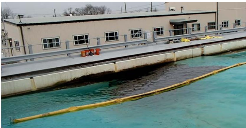
Figure 6. Waves varied in height throughout the experiments at Ohmsett; the waves made during Test 14 had a mean height of 15.9 Inches and wavelength of 39.8 Feet.
