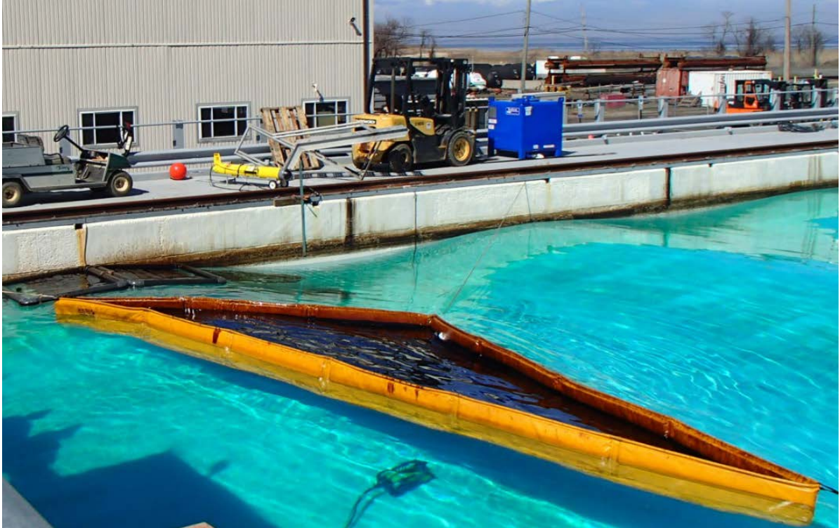
Figure 4. Upon collapsing to its minimum surface area, the arbitrary boom slick allowed measurements of a thicker slick.
