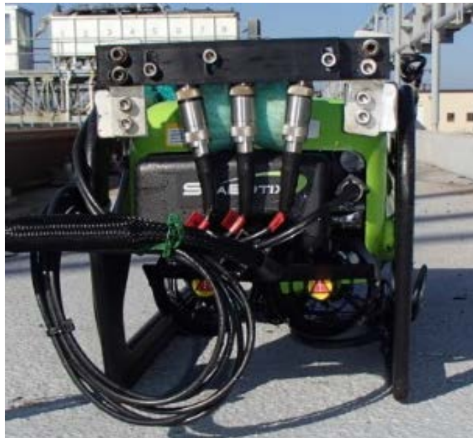
Figure 18. Side, top, and back views of the ROV showing the placement of the acoustic transducers mounted at various angles to account for the pitch and roll of the ROV platform.
