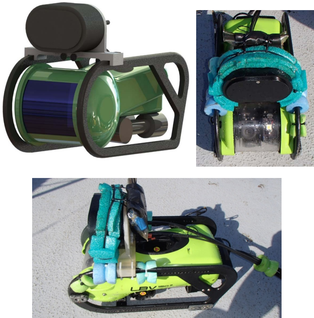
Figure 40. The large low frequency AirMar transducer was mounted on the ROV and floatation was added to ensure the ROV was neutrally buoyant. The high frequency acoustic measurements were performed using the two transducers mounted beneath the large AirMar low frequency transducer.
