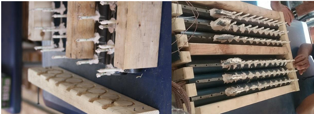
Figure 64: Thermocouple tower transportation housing showing tower-end sockets (left) and transport-ready configuration (left). During transport, the thermocouples would be facing down to prevent vibrational damage.
