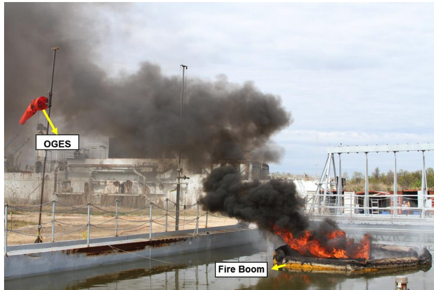
Figure 60: The Outdoor Gas Emission Sampling System (OGES) at Phase III
