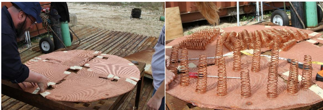
Figure 62: FR blanket prior to (left) and during assembly (right).
