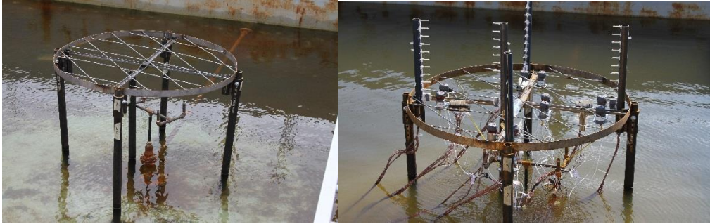
Figure 63: Burner assembly with legs only (left) and with full instrumentation including heat flux gauges, fuel layer thermocouples, and thermocouple towers, ~290 data points in all (right).
