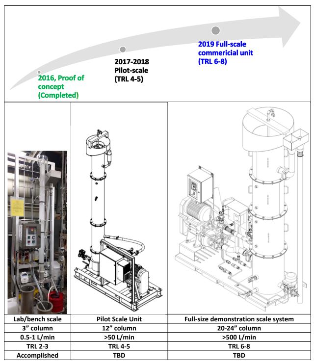
Figure 41. A scale-up process of flotation technology for oil spill response: Research, Development, and Demonstration.
