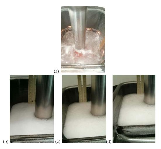
Figure 15. Gas holdup measurement in Denver cell: a) No frother, 1200 rpm, GH< 10 %; and 30 ppm of F672, b) 800 rpm, GH=14.5 %; c) 900 rpm, GH=25.9 %; and d) 1000 rpm, GH = 33 %, respectively.
