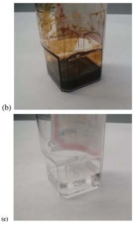
Figure 18a: (a) Oil flotation operating in a Denver cell; typical (b) crude sample, and (c) water sample collected from a Denver cell flotation operation, respectively.
