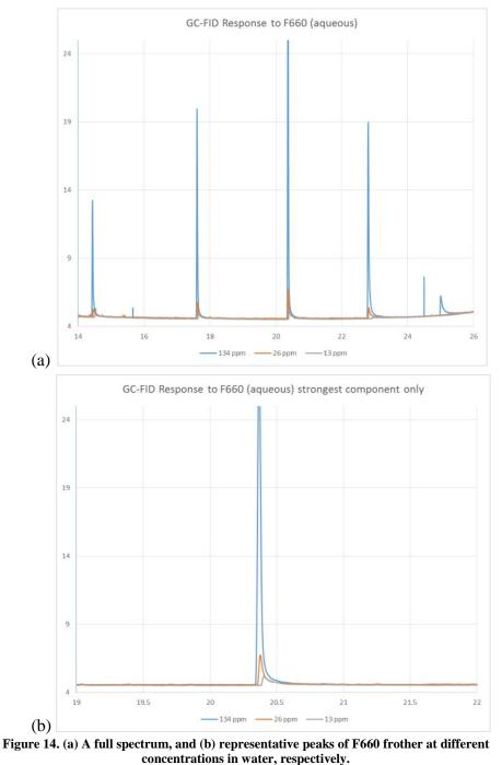
14b. However, salt compounds in seawater had strong impact on the FID, which failed quickly after seawater sample injection.
