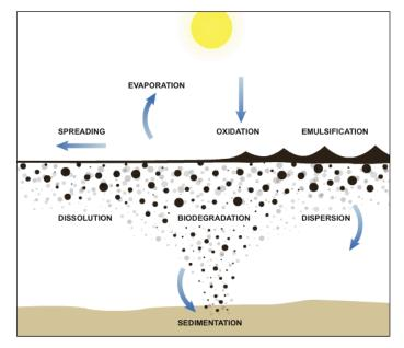
Figure 1. Schematic of oil spill dispersion process on sea (courtesy: Seapro.org).<sup>[1]</sup>
