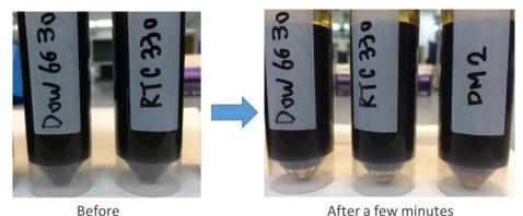
Figure 26. Water-in-oil emulsions (a) before and (b) after 120 seconds of adding 500 ppm of selected surfactants.
