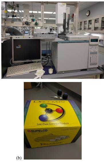
Figure 8. (a) Agilent 6890N gas chromatography, and (b) a SPE module, respectively.
