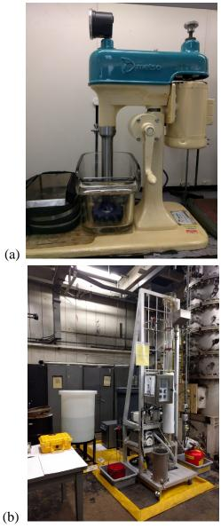
Figure 12. (a) A Metso Denver cell, and (b) an ErieZ 3" flotation column system, respectively.
