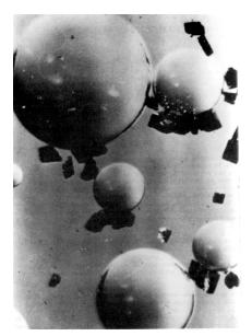
Figure 3. Attachment of fine particles on bubbles. <sup>[12]</sup>
