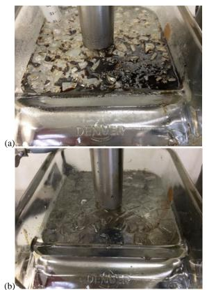
Figure 20. Oil contaminated ice (a) before and (b) after flotation in Denver cell. Ice size is 15 mm.
