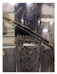
Figure 27. ANS crude in the presence of 10 ppm of Romax 6000 in flotation column at 5 °C.
