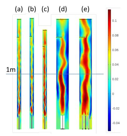
Figure 38. Liquid velocities of scale-up changes to the (a) initial column by (b) reducing flow, (c) reducing height, (d) increasing radius, and (e) multiplying spargers. The figure on the right is the legend in m/s.
