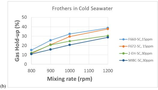
Figure 16. Performance of frothers in (a) DI water, and (b) seawater at 5°C, respectively.
