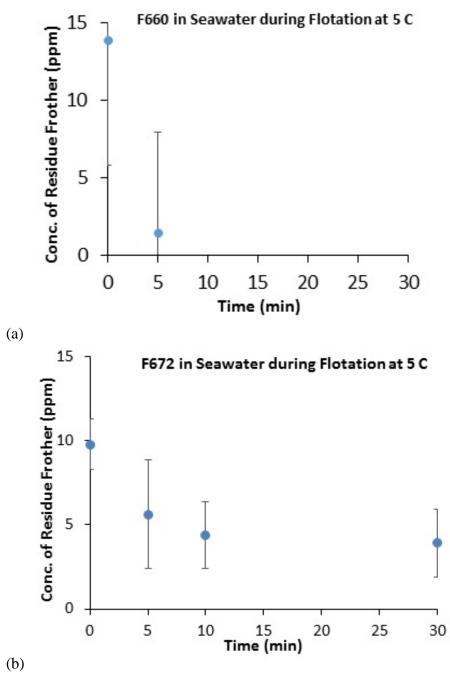
Figure 13. (a) Residual F660, and (b) residual F672 in seawater during flotation at 5 °C, respectively.
