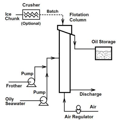
Figure 6. Flotation column system for oily ice water treatment.
