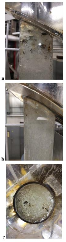
Figure 28. Oil contaminated ice (a) before flotation treatment, and (b) side view and (c) top view after flotation treatment in 3" column, respectively. (Baseline condition, ice particle size is 15 mm.)
