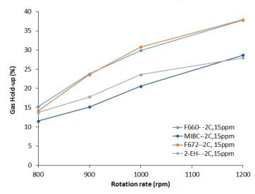
Figure 17. Performance of frothers in freezing seawater at -2°C.
