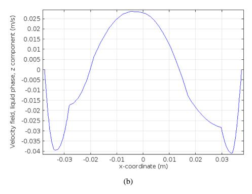
Figure 39. Water velocity profiles at 1 m height for (a) 1 L/min and (b) 0.2 L/min gas flow rate
