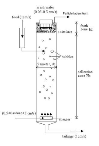
Figure 4. a) Schematic diagram of a conventional flotation cell, and b) a flotation column, respectively.
