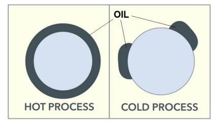
Figure 5. Oil air bubble interaction at different temperatures (courtesy: oilsandsmagazine.com). <sup>[18]</sup>
