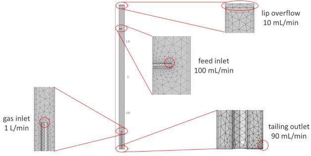
Figure 37. Base column model for COMSOL simulations
