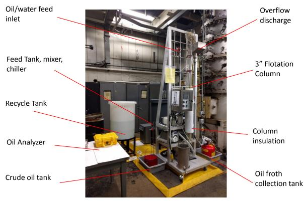
Figure 21. A 3" flotation column system for oil separation study.
