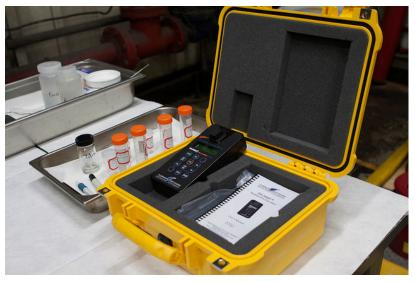
Figure 7. A TD-500D oil analyzer.
