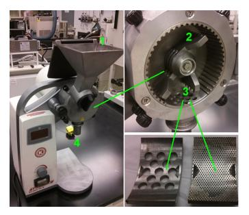
Figure 11. Laboratory hammer/cutting mill for solid sample grinding.
