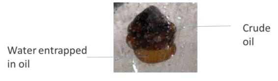
Figure 25. Water-in-oil emulsion was found in flotation operation.
