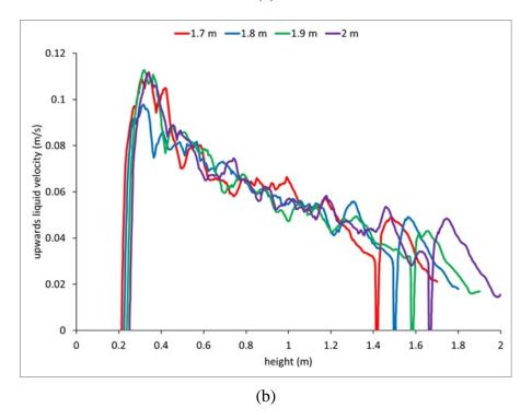
Figure 40. Water velocity profiles at (a) 1 m height for 3 column radii and (b) the centerline for 4 column heights Since these preliminary results are very useful for designing new floatation column and improving the efficiency of separation, further simulations should be focused on pilot-scale level to optimize the column size, to design the flexible column head used onboard, and to explore the effective inlet fluid flow pattern for high separation performance.
