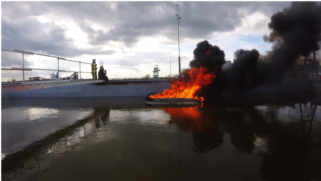
Figure 3.10. ANS/Aggregator 13:1 Ratio Burn (B7) at JMTF. A 13:1 ratio of ANS crude oil and PNNL aggregator were used in this burn test.
