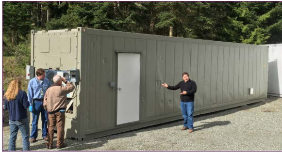
Figure 5.1. Freezer Laboratory. The freezer laboratory at MSL operates at air temperatures down to -15°C. A closed looped chiller line operates -30°C. The laboratory is highly flexible, can be fitted with a variety of tank types and sizes, and is permitted to operate with crude oil and dispersants.
