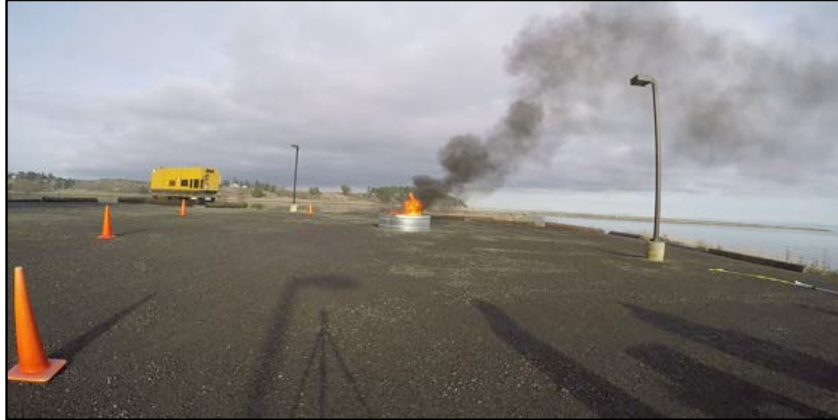
Figure 2.20. Large-scale burn of 3.0 L of Dorado crude without aggregator in ice /seawater.
