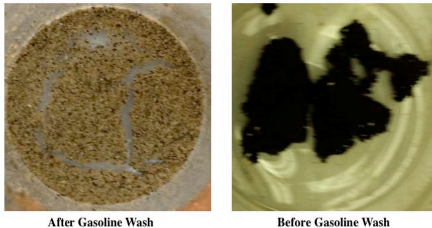
Figure 3.14. Dorado Tar Residue Before and After Solvent Extraction. A sample of the Dorado tar residue was washed with a gasoline solvent to remove tar and oil residue from the sample to determine if there was any remaining aggregator or wood flour base product remaining in the post-burn sample. The post wash sample showed the presence of a wood product similar to the aggregator-only control.
