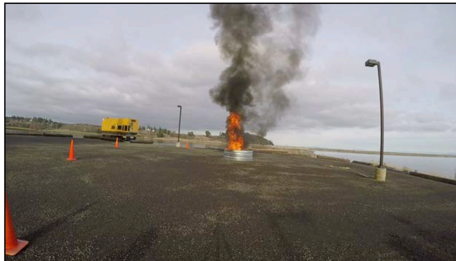
Figure 2.21. Large-scale burn of 3.0 L of Dorado crude with 180.0 g of aggregator in ice /seawater.
