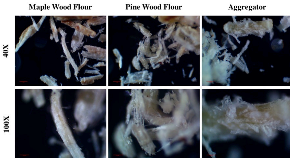
Figure 4.7. Representative microscopic pictures (30°C, 8 Weeks). The maple and pine wood flour samples were mixed with a H. resinae spore suspension and the aggregator was mixed with all three oil-degrading microorganisms ( A. borkumensis , P. putida and H. resinae ).
