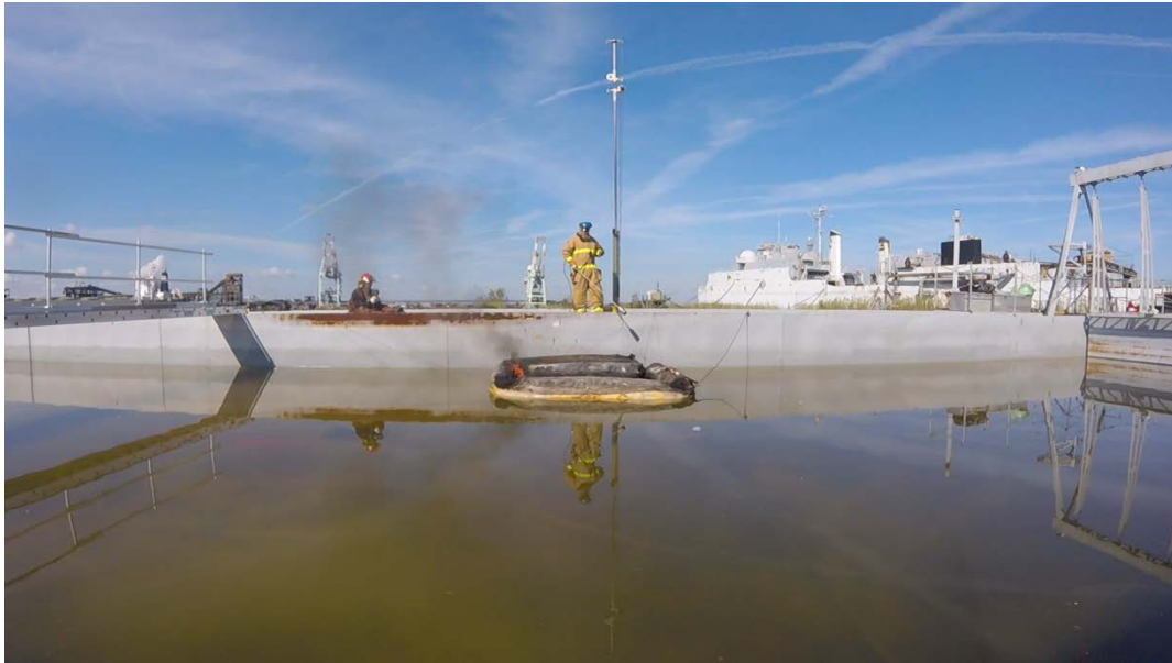
Figure 3.7. Dorado/Aggregator 10:1 Ratio Burn (B5) at JMTF. The picture is from burn five (B5). A 10:1 ratio of Dorado crude oil and PNNL aggregator were used in this burn test. Crude oil was placed on water and left overnight to weather oil.
