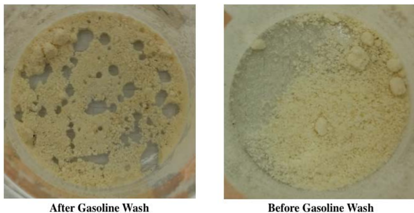
Figure 3.12. Aggregator-Only Before and After Gasoline Wash. The aggregator-only was used as a control to compare with the ANS and Dorado post-burn tar residue samples from the JMTF test burns.
