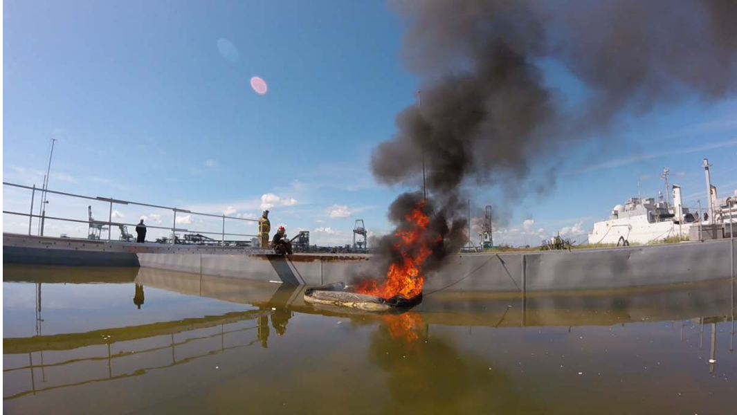
Figure 3.5. Dorado/Aggregator 10:1 Ratio Burn (B4) at JMTF. A 10:1 ratio of Dorado crude oil and PNNL aggregator were used in this burn test.
