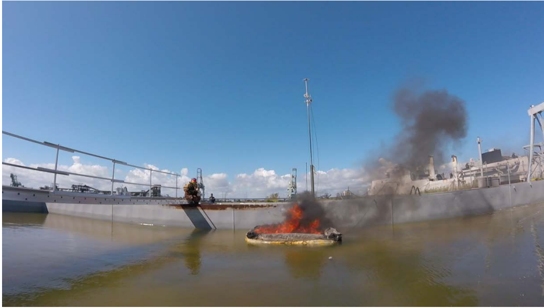
Figure 3.1. Dorado/Aggregator 3:1 Ratio Burn (B2) at JMTF. The picture is from burn two (B2). A 3:1 ratio of Dorado crude oil and PNNL aggregator were used in this burn test. Image was taken using a GoPro camera.
