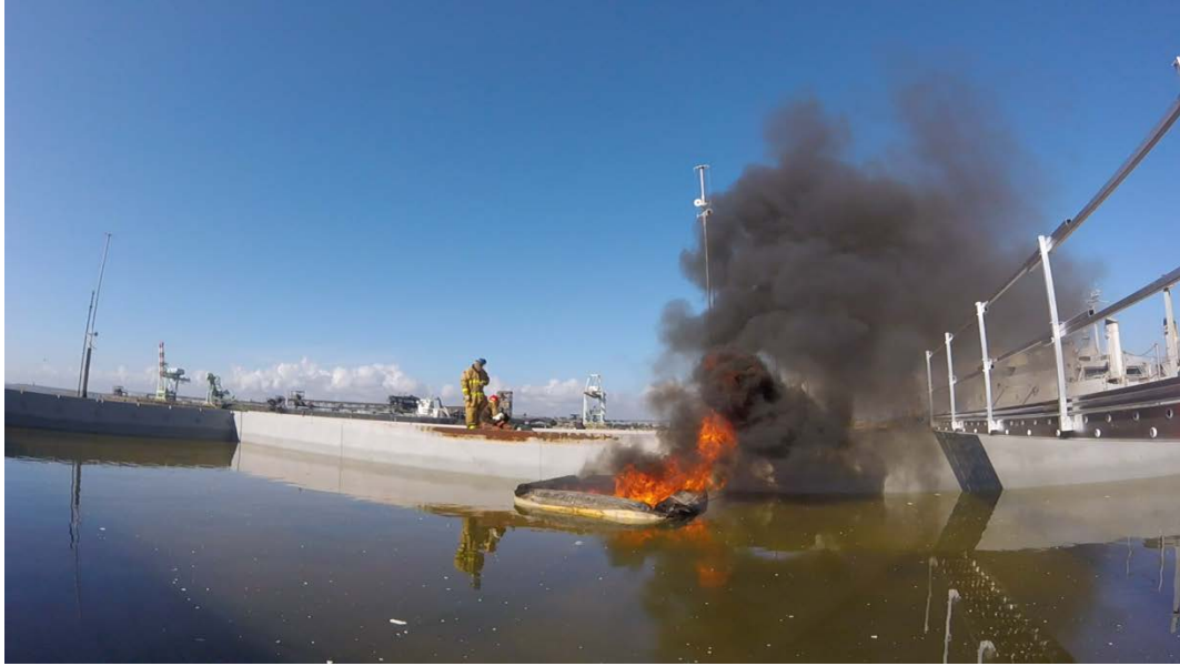
Figure 3.3. Dorado/Aggregator 11:1 Ratio Burn (B3) at JMTF. The picture is from burn three (B3). A 11:1 ratio of Dorado crude oil and PNNL aggregator were used in this burn test.
