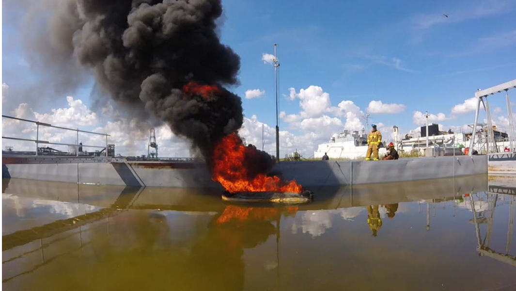
Figure 3.8. Alaskan North Slope (ANS)/Aggregator 6:1 Ratio Burn (B6) at JMTF. A 6:1 ratio of ANS crude oil and PNNL aggregator were used in this burn test.
