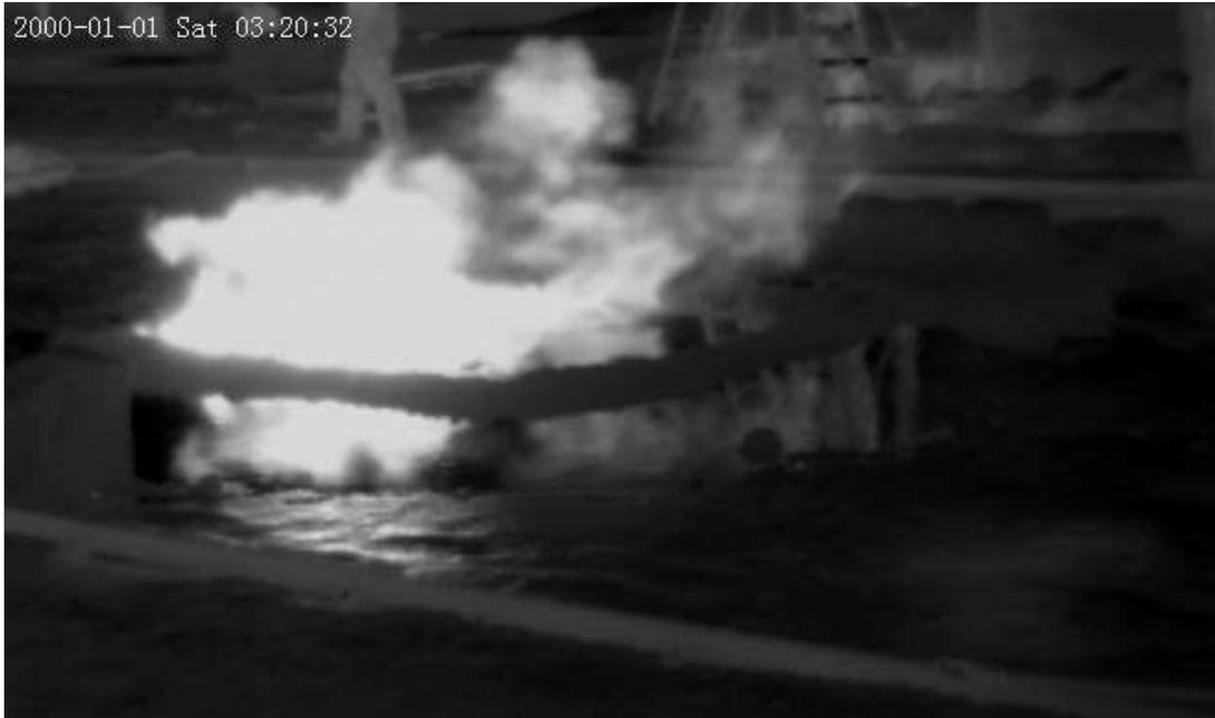
Figure 60. IR image shows reflection and smoke. The fire and smoke blend together because they both go over the upper threshold for the uncooled long wave IR.
