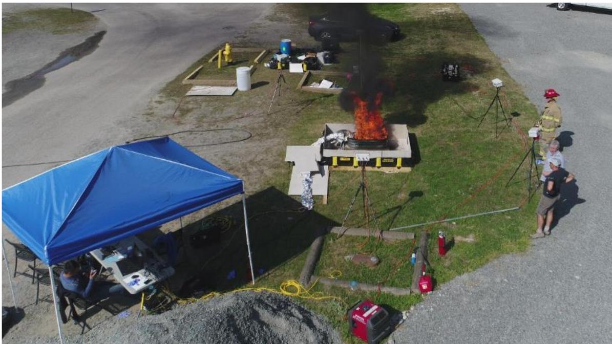
Figure 3. Outdoor burning setup at ARA VIMS facility. Photo: Donglai Gong
