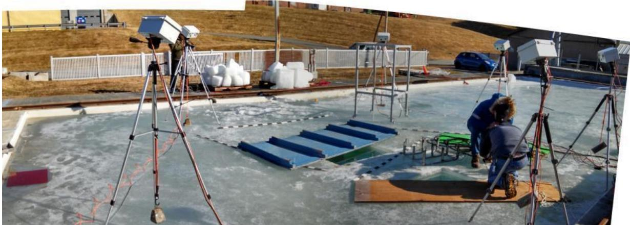
Figure 53. White camera enclosures on tripods prior to testing at the CRREL ice facility. The frame to hold the transducers is behind the blue board.
