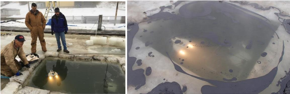
Figure 82. The ROV in the water (left) and the oil residue left after burning ANS in the ice field (right).
