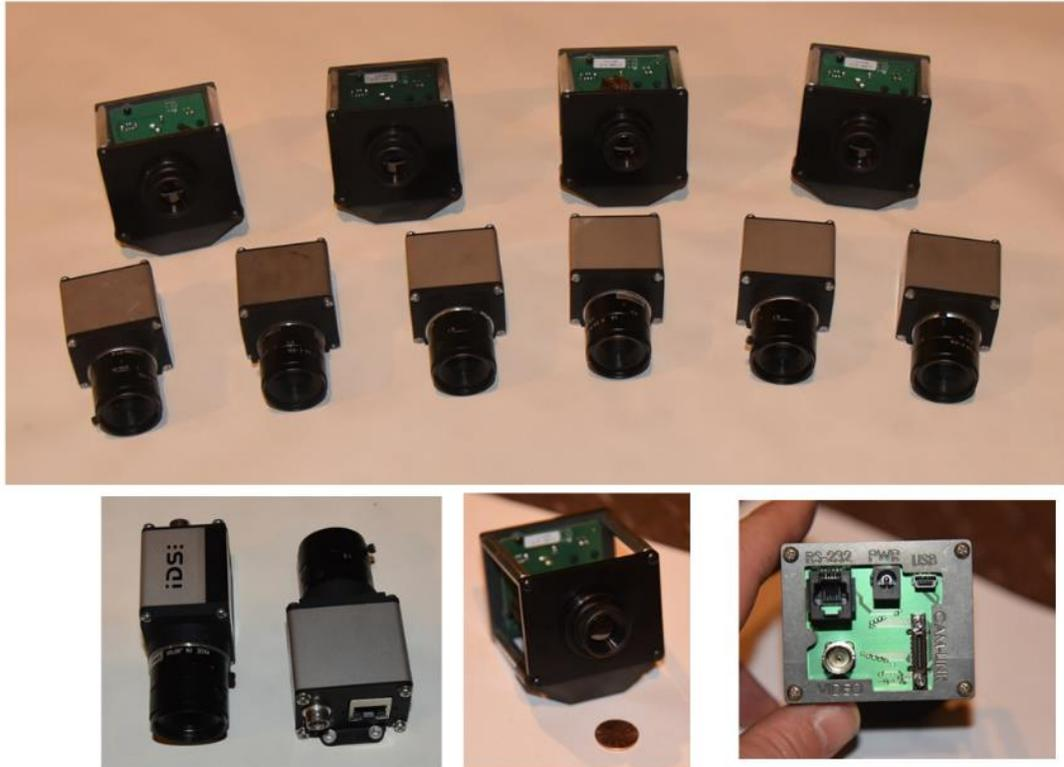
Figure 6. Visible and infrared (IR) cameras.
