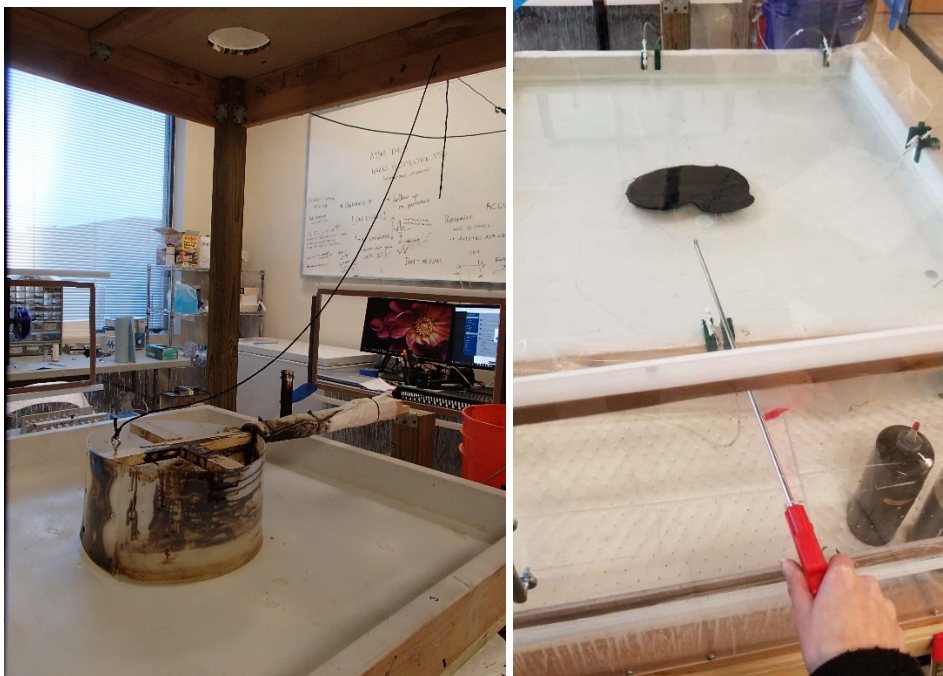
Figure 3: oil containment ring left, tube with low volume air flow right
