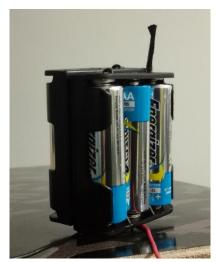
Figure 93: 9V Battery Pack - AA Batteries
