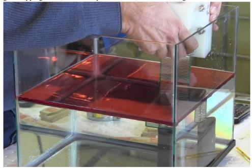
Figure 116: Experimental setup for dipping tests (Ohmsett)
