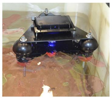
Figure 138: LED-based Sensor - Diesel Test (Tank)
