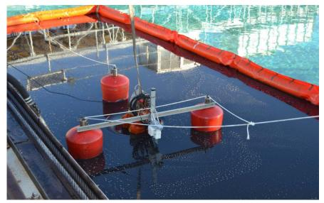
Figure 133: Sensor #1 Mounted to Desmi Termite Skimmer
