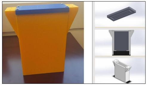
Figure 28: Capacitive Sensor Packaging - Prototype 1
