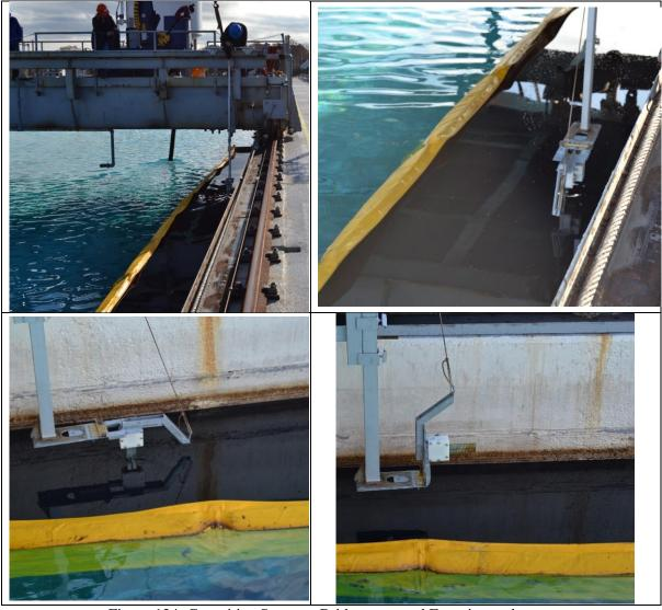
Figure 124: Capacitive Sensor – Bridge-mounted Experimental setup
