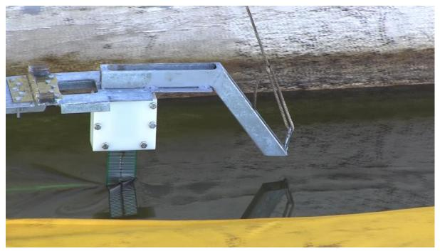
Figure 126: Bridge-mounted Sensor while dragging (Snapshot from video# 00131)
