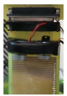
Figure 86: Capacitive sensor with vibration mechanism
