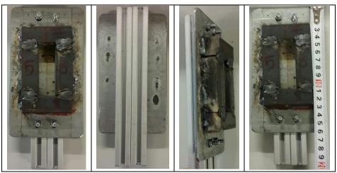
Figure 113: Manufactured skimmer mount sensor holder
