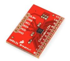
Figure 24: MPR121 Breakout Board
