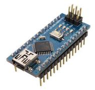
Figure 8: Arduino Nano Board
