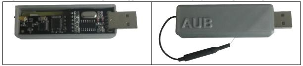
Figure 10: Wireless-to-USB receiver module
