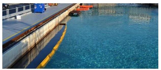
Figure 127: Photo showing boom bellying outward
