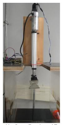
Figure 48: Capacitive Sensor Experimental Testbed - Lab tank
