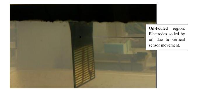
Figure 81: Photo showing oil-fouled electrodes
