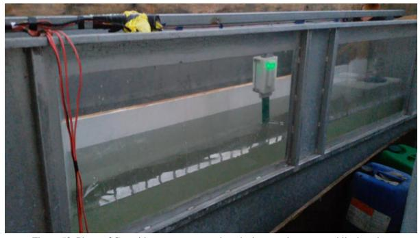
Figure 58: Photo of Capacitive sensor mounted on the large tank actuator while dragging
