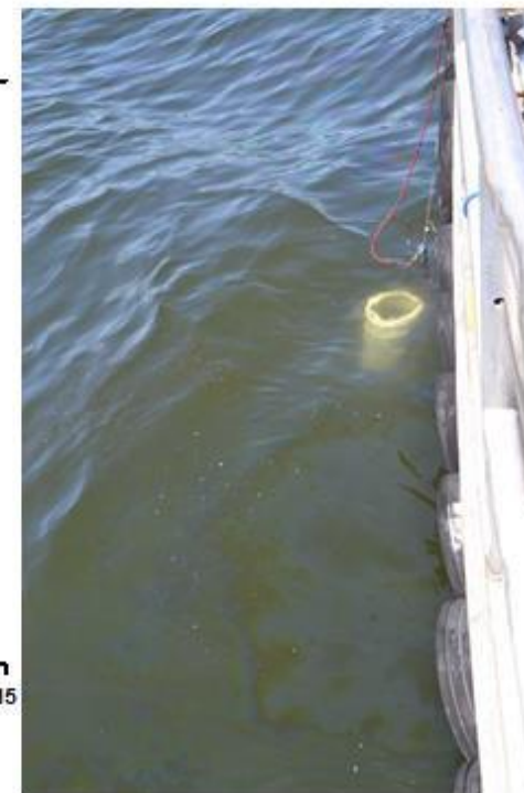
Figure 3.45. UV light penetration to 1.3–1.5 m on April 25, 2017 beginning at 1:45 p.m. The Biospherical radiometer (submerged white container in photograph) measured light intensity at various wavelengths, while contained in a protective housing with a UV-transparent lid. The radiometer was deployed upwind of the surface slick and attached to the side of the boat as the boat drifted into the slick. The photograph, showing the radiometer below the surface sheen, was taken approximately 10 minutes and 23 seconds into the drift (dashed vertical line on plot). Waypoint (WP) numbers are also shown on the plot to mark the beginning of the sheen and other observations regarding slick thickness or boat shadows that were observed during the transect. The protective housing caused shadows and other interferences; therefore the data presented here represent a trimmed subset that did not contain these anomalous values.
