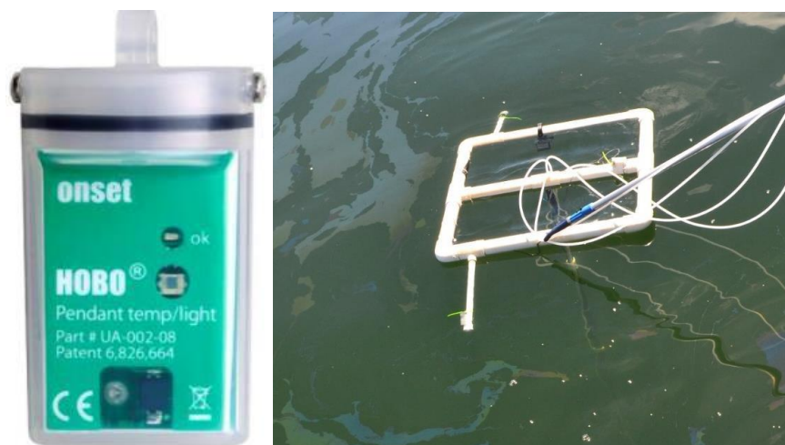
Figure 2.7. HOBO light and temperature sensor/logger and water collection raft with GoPro camera and HOBO sensors attached to the submerged arms and air-exposed middle section (August 2017).
