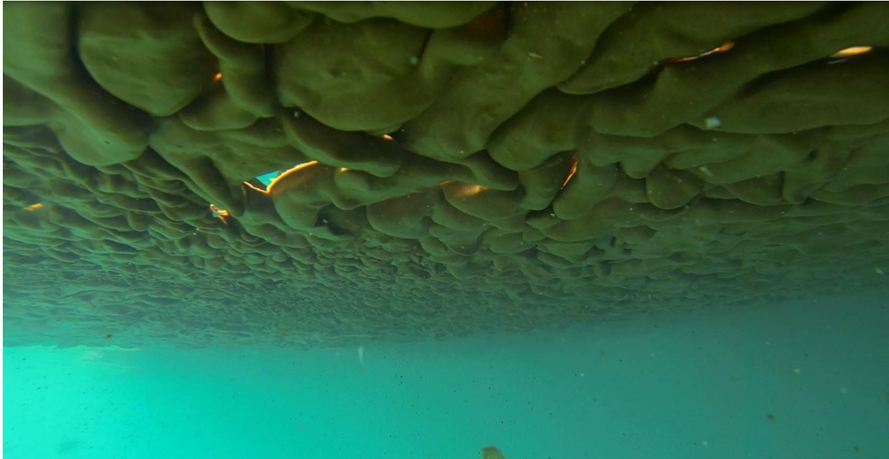
Figure 3.20. Photograph taken underneath the Ohmsett oil slick, demonstrating the heterogeneity of the emulsified oil.
