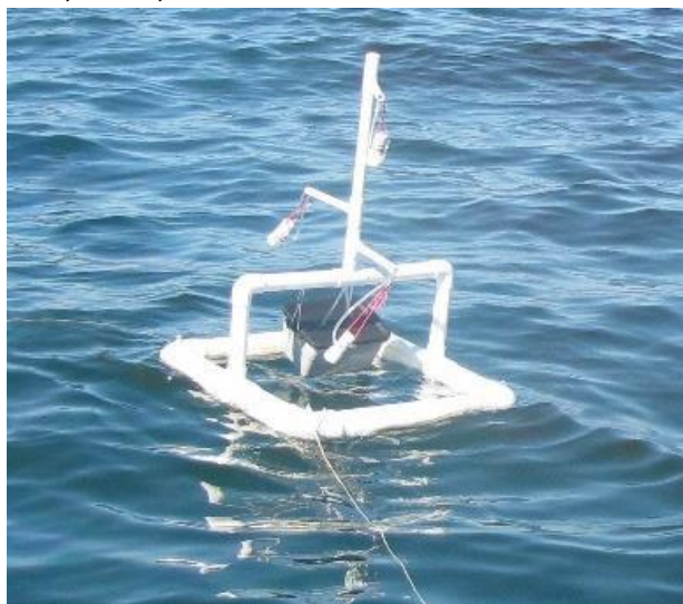
Figure 2.8. Floating air sampler that collected samples at 0.1 m, 0.5 m, and 1.0 m off the surface of the oil slick.
