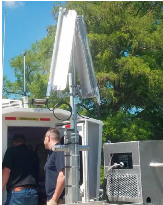
Figure 2.9. RF antenna that Ocean Imaging and MSRC installed on the boat for the April 2017 sampling. This allowed direct data communications between the King Air carrying TRACS and the boat at MC20.
