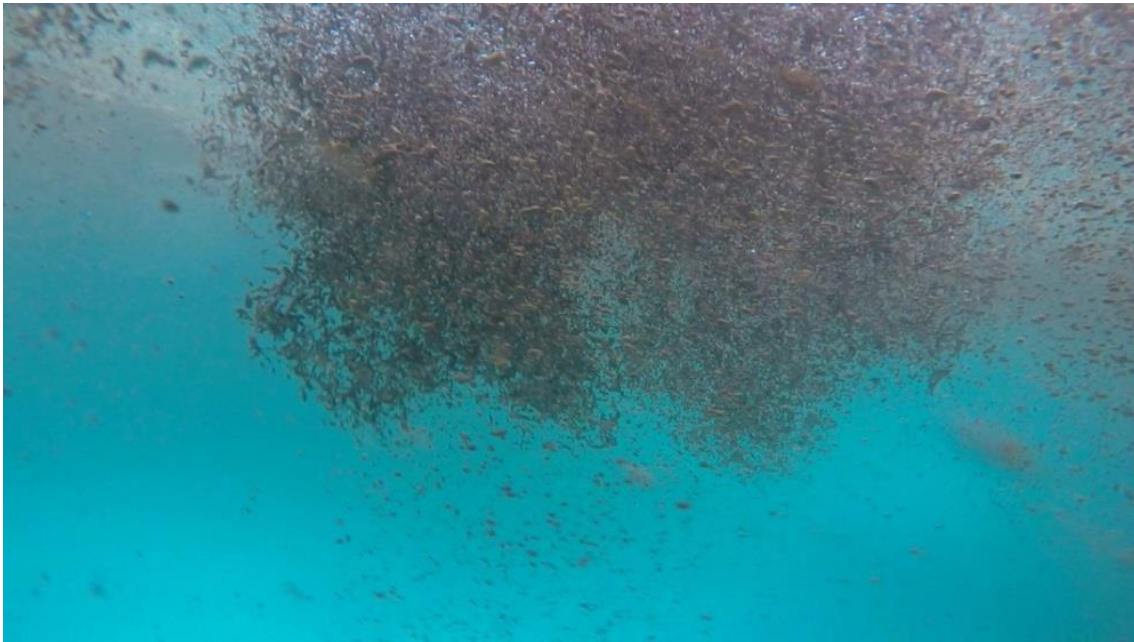
Figure 3.28. Oil droplets mixing into the water column and emulsifying after the wave generators started at Ohmsett. The photograph was taken from an underwater observation window.
