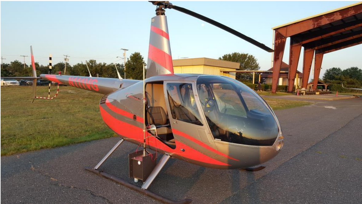
Figure 2.3. TRACS sensors mounted to a vertical pole on a Robinson R44 helicopter.
