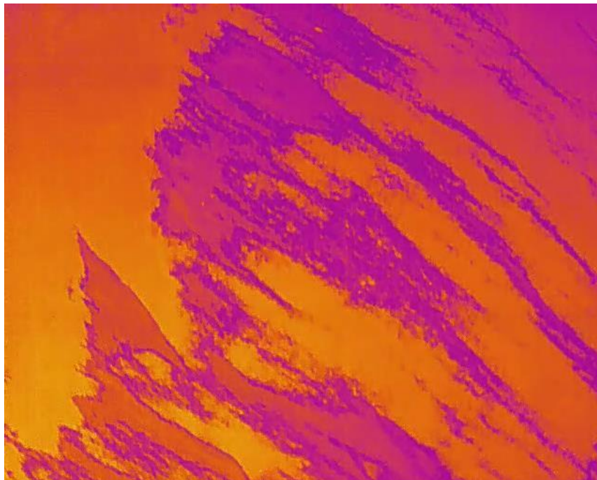
Figure 3.5. FLIR thermal IR image of the MC20 oil slick on November 15, 2016. This image was collected shortly after the image in Figure 3.4, at a lower altitude. Thicker oil appears darker.
