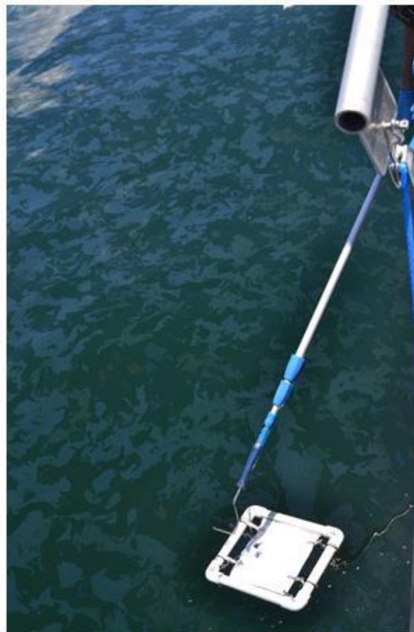
Figure 3.48. Water parameter profiles collected with the YSI datasonde near MC20 on August 17, 2017 at 12:26 p.m. The oil sheen is visible on the surface while a sorbent pad is used to collect oil at the same time. The sonde collected data continuously as it was lowered to a depth of about 17 m and then brought back to the surface.
