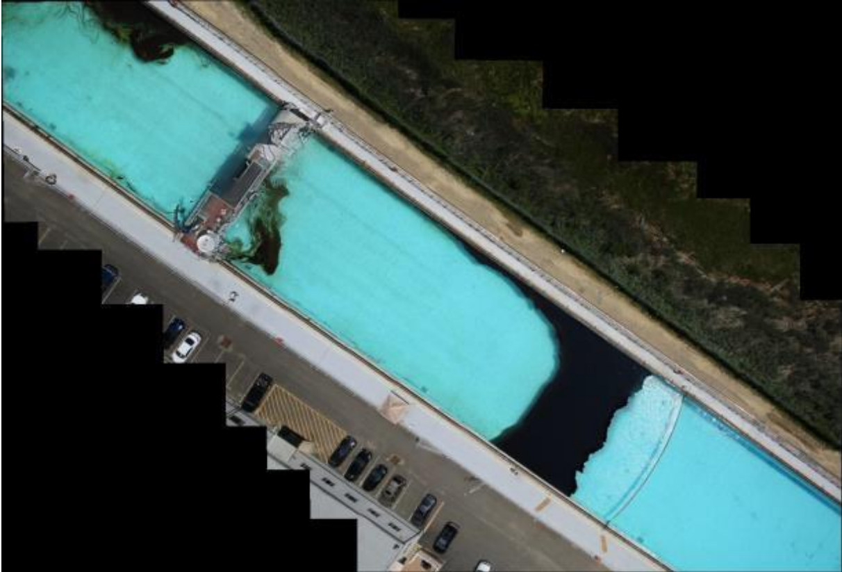
Figure 3.1. Orthorectified mosaic image of the oil slick at Ohmsett, collected using the HD camera mounted on a DJI S1000 drone.
