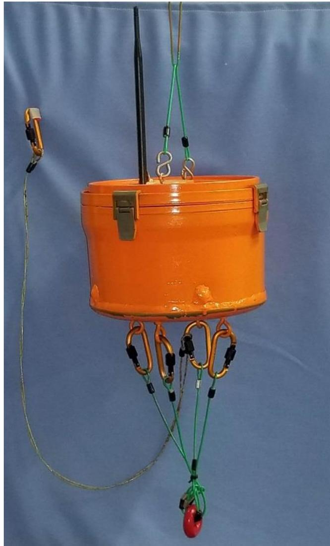
**Figure 3-4: WCM-Buoy enclosure with external antennas and counter-balance weight**
