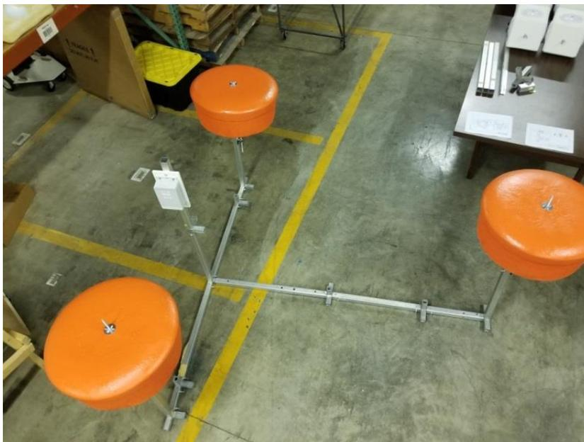
**Figure 3-9: Mock weir skimmer with WCM-embedded software development platform**
