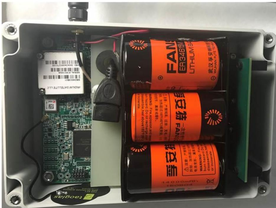
Figure B-3: Installed WCM-Sat batteries
