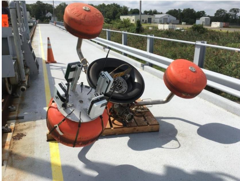
**Figure 4-3: Two WCMs, WCM-Sat, and WCM-embedded software development platform mounted to one of the Desmi Terminator's floats**
