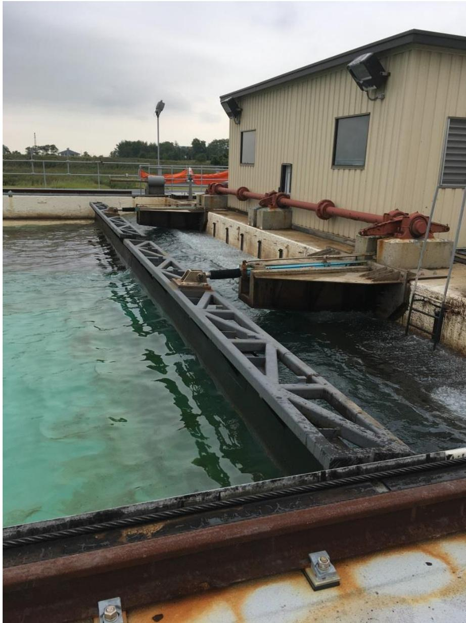
**Figure 4-2: Ohmsett wave generator**
