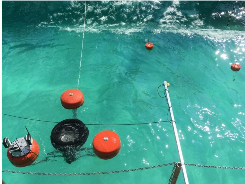
Figure 4-5: Skimmer and WCM-Buoy deployments looking down from the auxiliary bridge
