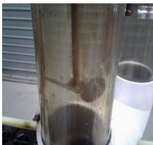
Figure 4. Impeller used to force oil-water mixture flow.
