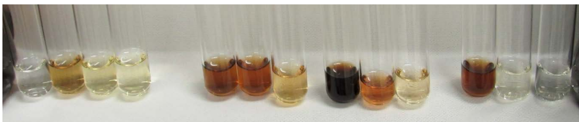
Fig. 4-Eluent from each of the solvent washes during the SARA separation. They are arranged, from left to right, as saturates, aromatics, resins, and asphaltenes.
