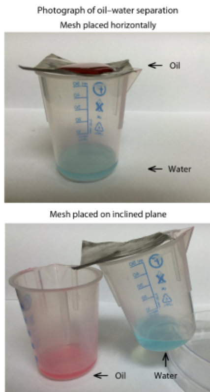
Figure 4-5. Laboratory experiments confirm that multi-layered coated mesh is effective in separating oil and water both in a pour-through configuration and on an inclined plane (Solomon et al., 2014)
