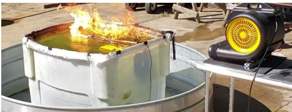
Figure 8 Wind Test Ignition at 18 kts
