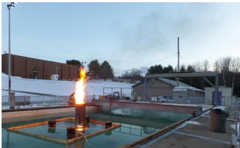
Figure 4: Floating burner tests at CRREL.
