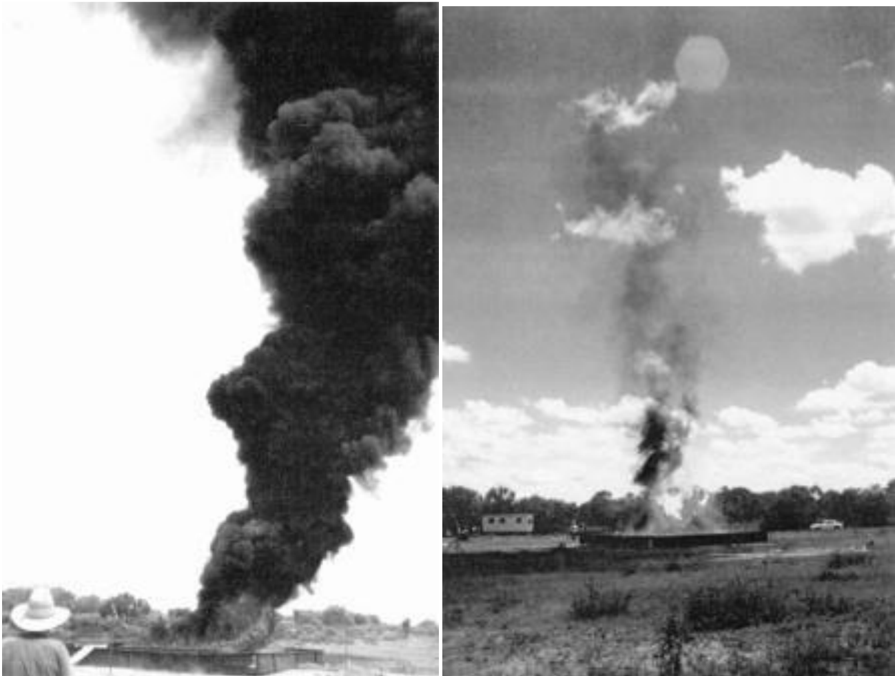
Figure 34. MSRC burn tests without and with aeration
