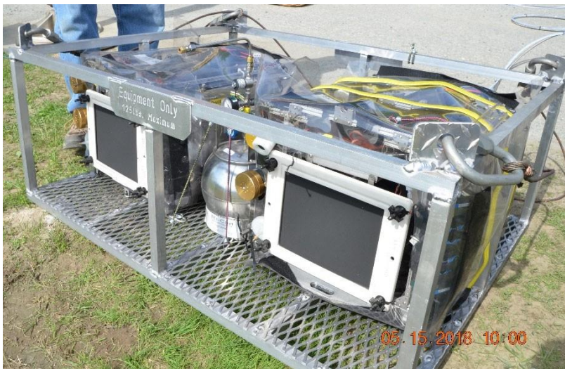
Figure 2-2. U.S. EPA's emission instrument system mounted on an aluminum skid.
