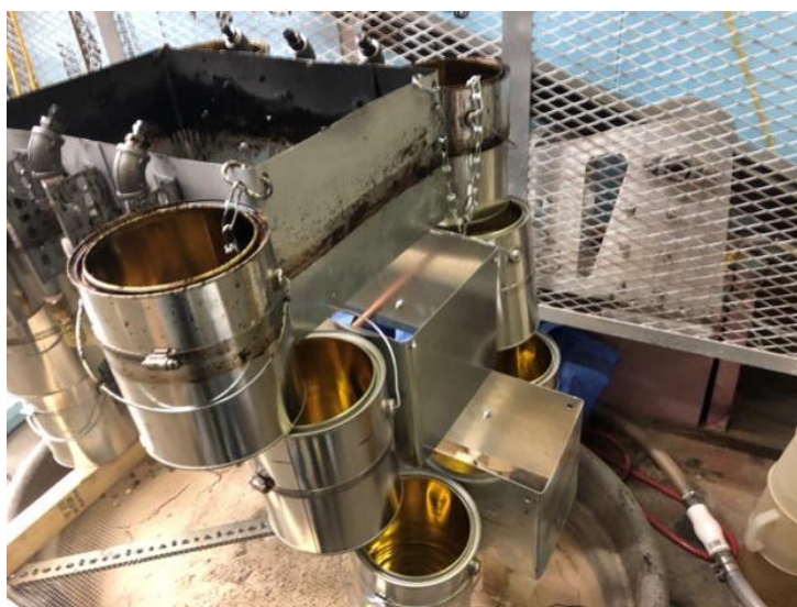
Figure 9: Comparison of fire boom models with different aspect ratios.
