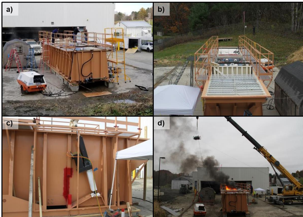
Figure 17: CRREL wave tank a) Air compressor and deluge water cooling pump, b) View from wave paddle end, c) Wave actuator, d) EPA smoke sampling package suspended by crane being moved into position.
