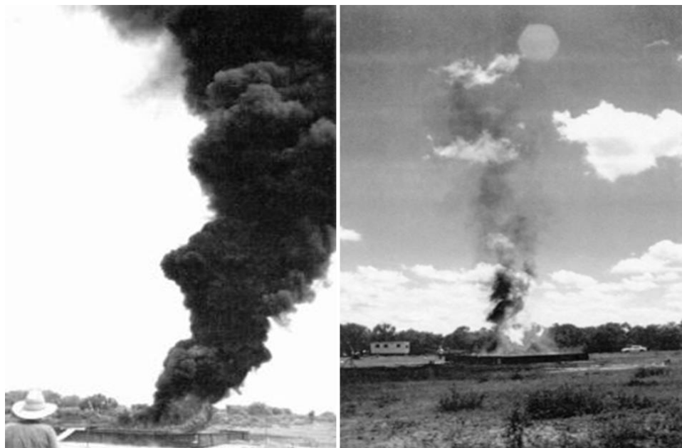
Figure 3: MSRC burn tests without and with aeration.
