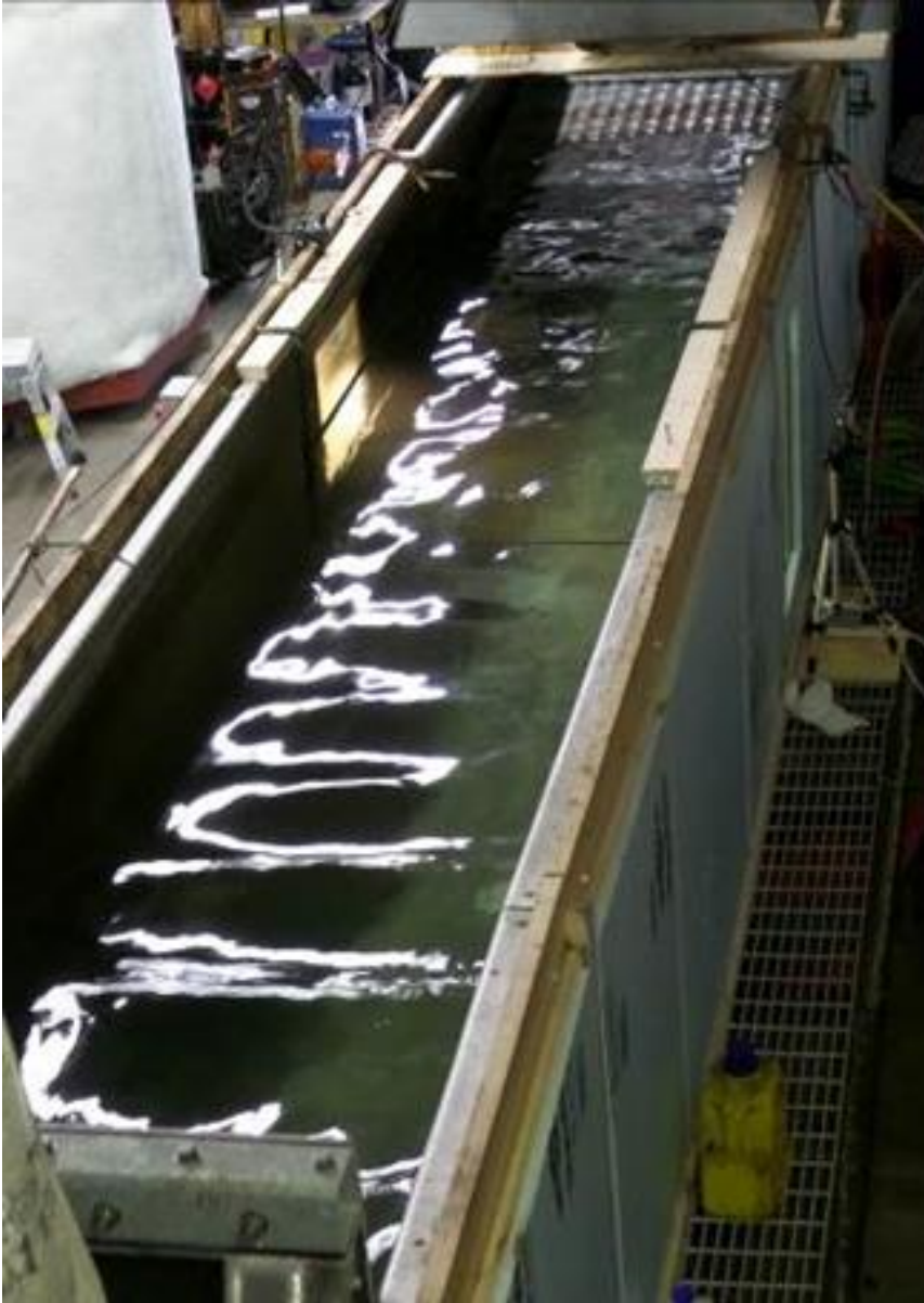
Figure 7 - Example of waves in the SL Ross wave tank.
