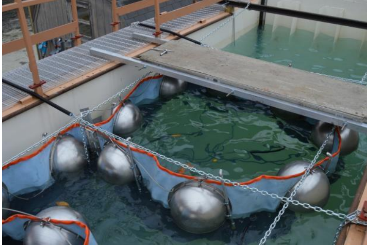
Figure 16: PyroBoom® with air nozzles deployed in CRREL wave tank. Note chains attached to large springs to hold PyroBoom test section in place yet allow movement in waves. Also note compressed air hoses retained underwater.
