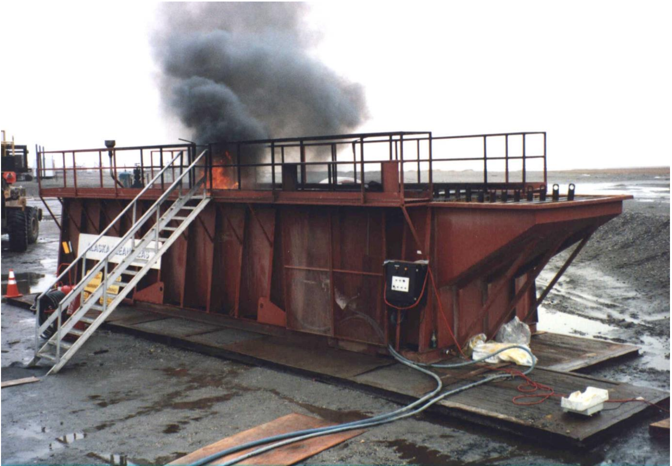
Figure 46 – Photo of original ACS wave tank showing burn test being conducted in Prudhoe Bay. This tank has been obtained by CRREL and shipped to Hanover for refurbishment.
