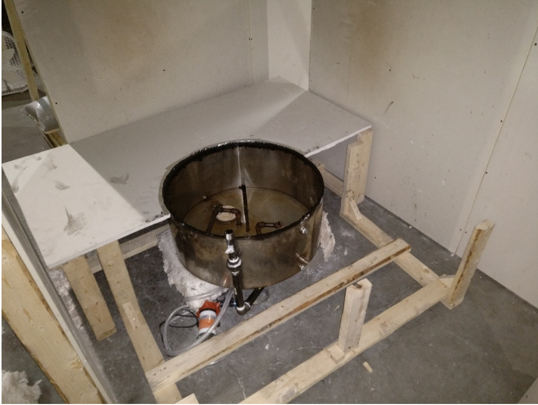
Figure A4. Fuel/water container shown here positioned in the center of the enclosure. The enclosure base was partially removed to show the support frame.
