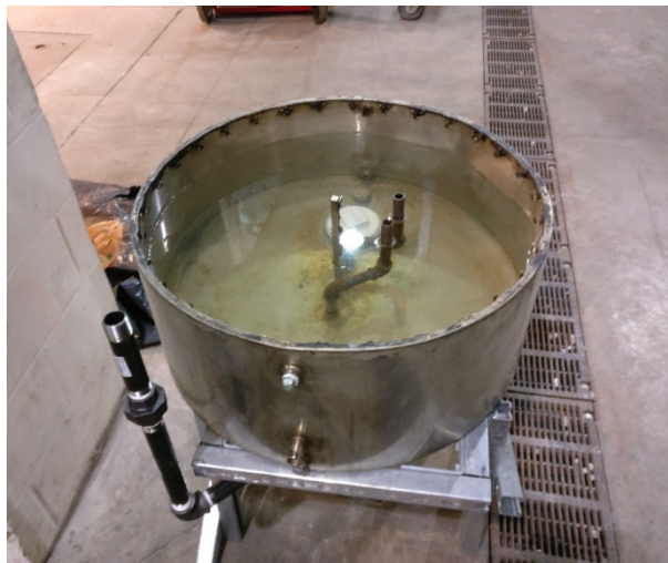
Figure A3. Fuel/water container being tested for leaks. Also visible are the inlet/outlet ports for water recirculation, and the scape pipe for running instrumentation wires.
