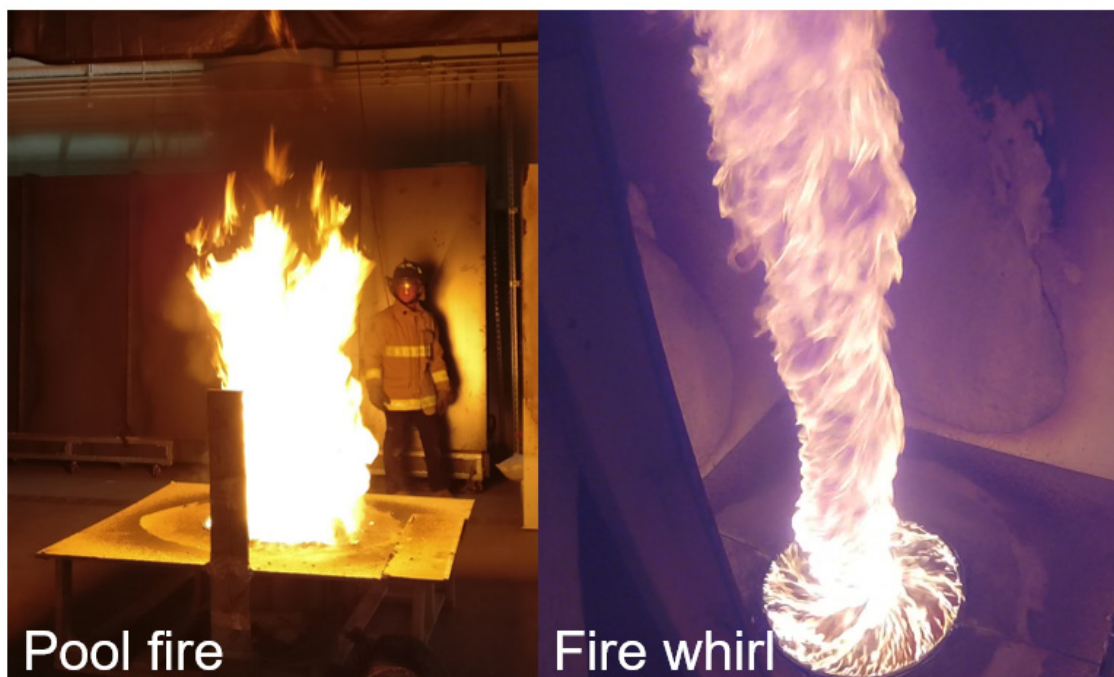
Figure 7.3: Images of ANS crude oil pool fire (left) and fire whirl (right). The image of the pool fire was obtained with a roughly horizontal view, while the image of the fire whirl was obtained looking down from the top of the walls due to the limited visual access around the walls.
