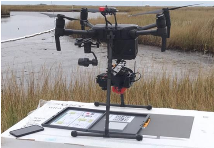
Figure 26. Multispectral UAS system pre-flight calibration steps.
