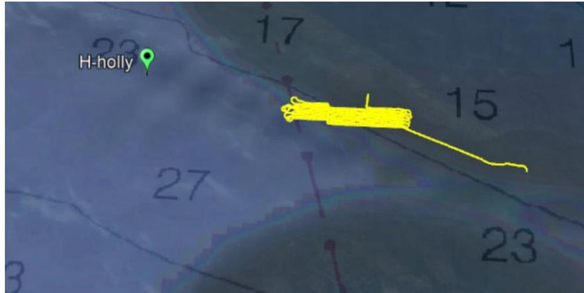
**Figure C.64. FDOM and optical backscatter measurements along the REMUS-100 vehicle track (top) for Mission 5.** Colors correspond to concentration. Scatter plot of optical backscatter as a function of FDOM (bottom). Chlorophyll concentration is indicated by symbol size. Colors correspond to depth in the water column.
