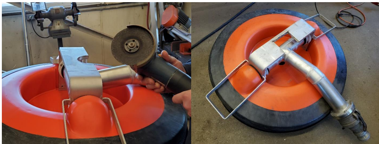
Figure 6: On the left, DESMI Minimax prior to modification. On the right, DESMI Minimax after modification to allow further angular rotation.
