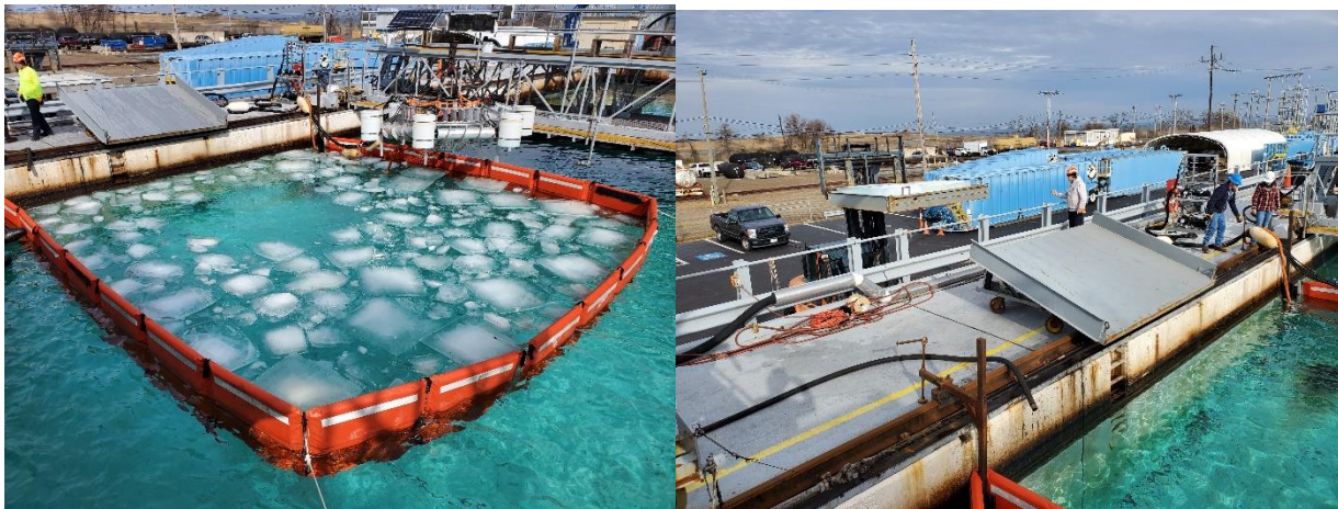
Figure 2: On the left, 70% ice field. On the right, ice delivery slide.
