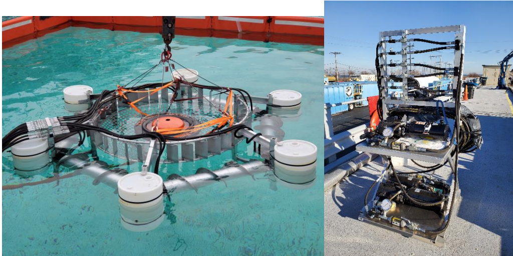
Figure 3: On the left, AIMS auger configuration. On the right, AIMS hydraulic power control system.
