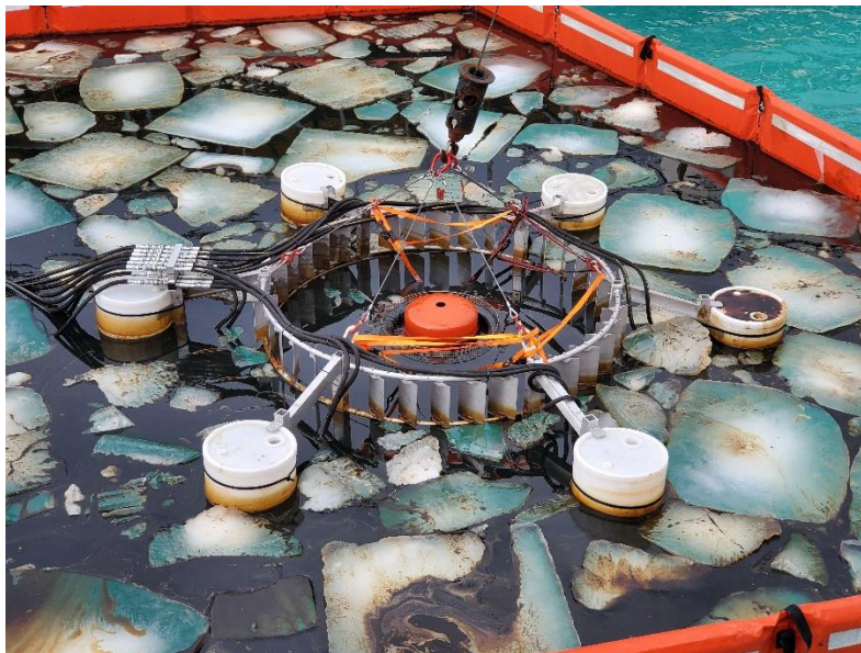
Figure 7: AIMS deployed in ice field with 1-inch oil slick.
