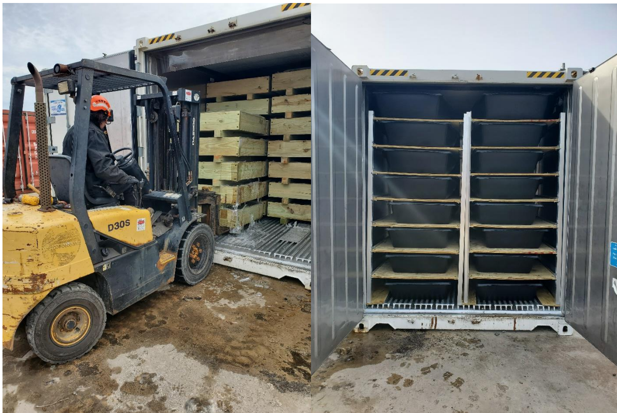
Figure 1: On the left, wooden ice forms in reefer. On the right, plastic ice forms in reefer.
