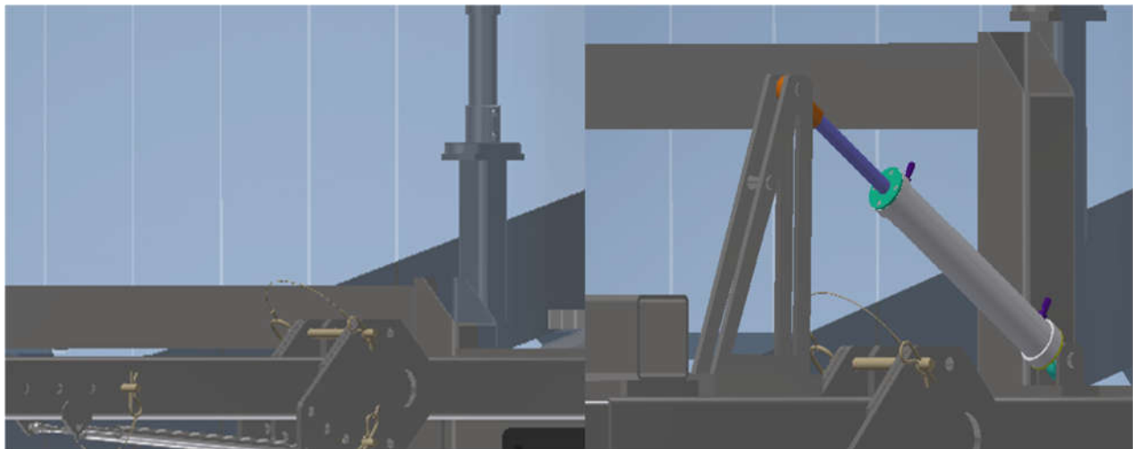
Figure 33. Proposed hydraulic actuator system on right, existing configuration on left.
