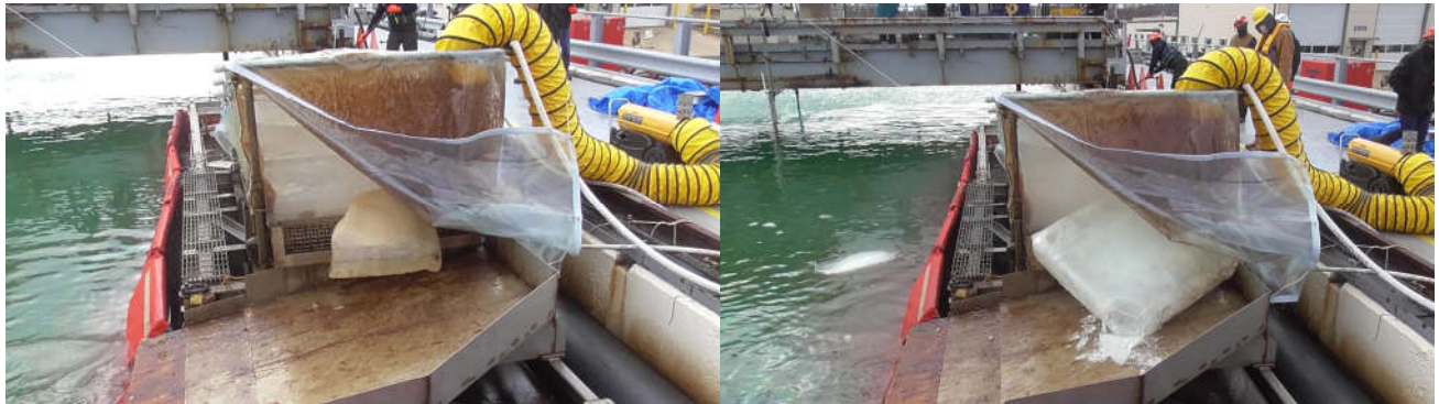
Figure 26. 60 psi spray test – 1 top spray bar on left, 3 on right.
