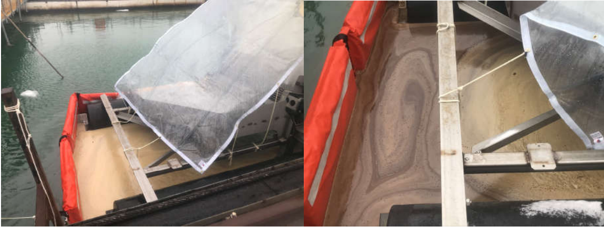
Figure 28. Hydrocal emulsion after 90 psi (left) and 30 psi (right) January 26.
