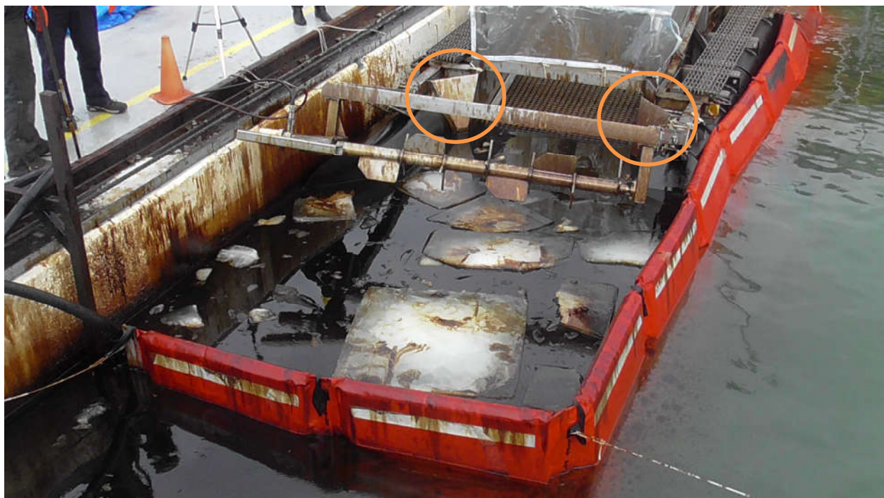
Figure 15. Front view of BOWHEAD in static configuration pool of weathered HOOPS. Chamfered sidewalls are circled.
