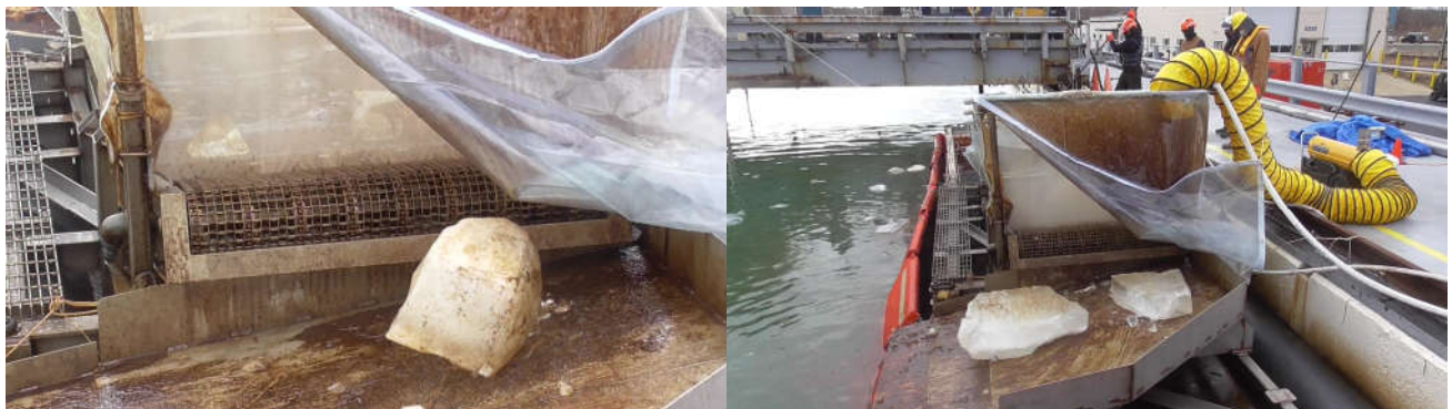
Figure 27. 30 psi spray test – 1 top spray bar on left, 3 on right.
