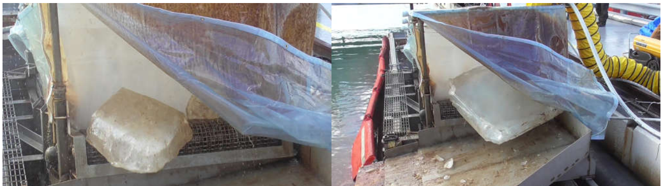
Figure 25. 90 psi spray test – 1 top spray bar on left, 3 on right.
