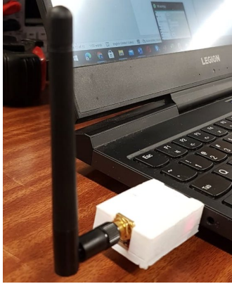
Figure 3.45: Wireless Module supporting USB connection on Laptop.
