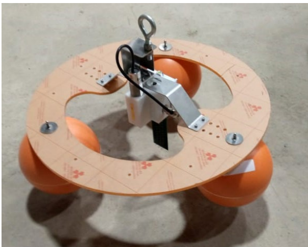
Figure 2.78: Floating configuration for the handheld sensor
