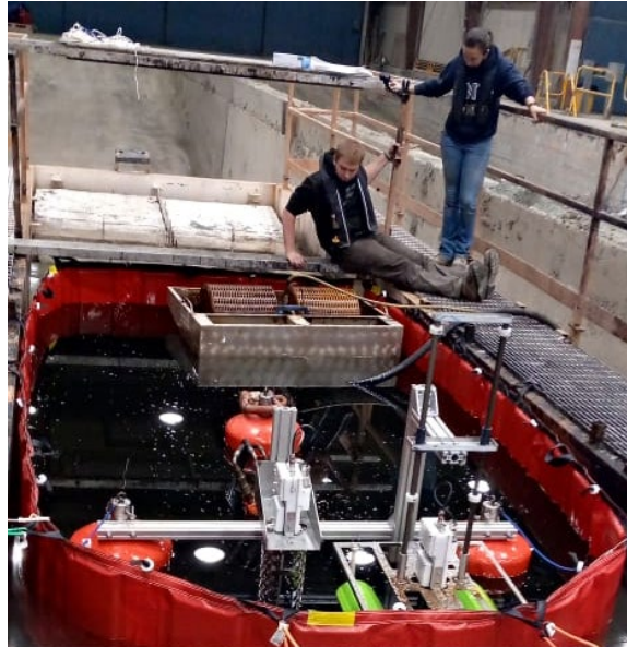
Figure 6.6: Skimmer placed behind the Termite to remove the oil
