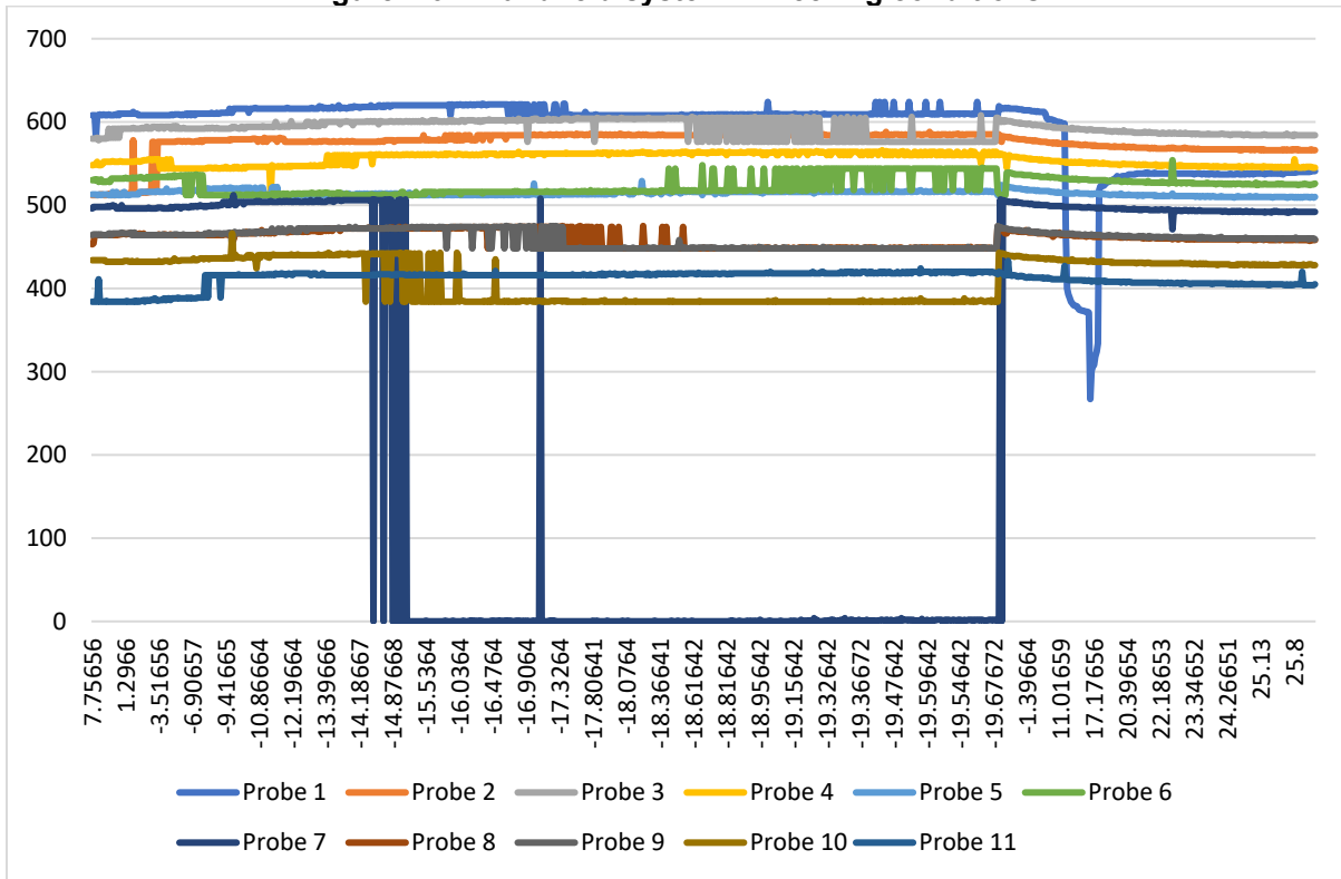
Figure 2.65: Capacitive touch values vs temperature.
