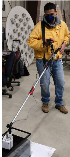
Figure 2.77: Handheld control unit and sensor mounted on the pole
