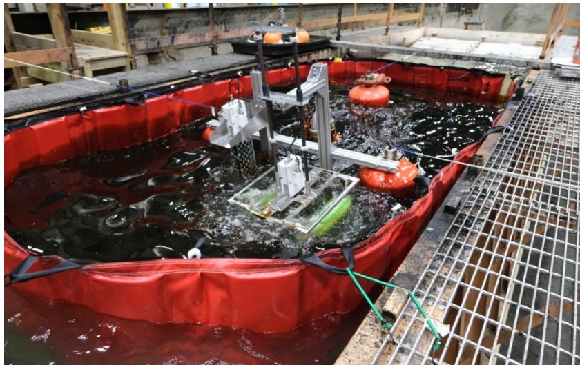
Figure 4.7: Skimmer with sensors in the enclosed area.
