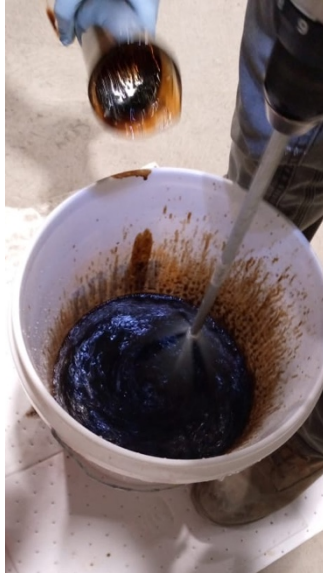
Figure 4.9: Emulsion mixing process.
