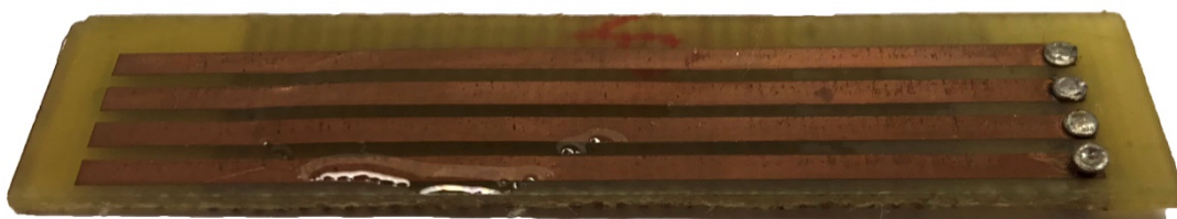
Figure 2.19: Water droplet completely wetting the surface of the sensor board piece coated with AcuWet ON-470
