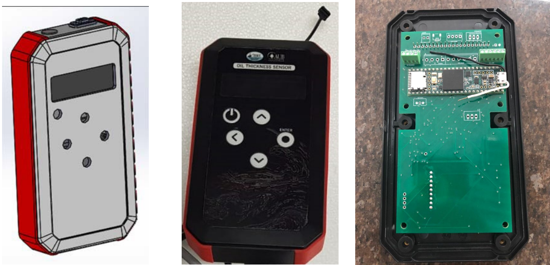
Figure 2.71: 3D and manufactured handheld enclosure
