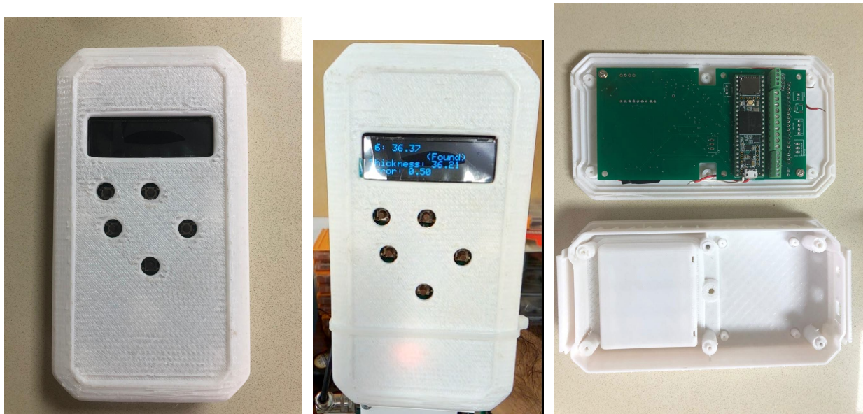
Figure 2.69: Handheld enclosure with assembled PCB
