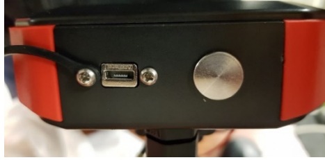
Figure 2.70: Top view of the handheld enclosure showing USB socket and temperature sensor
