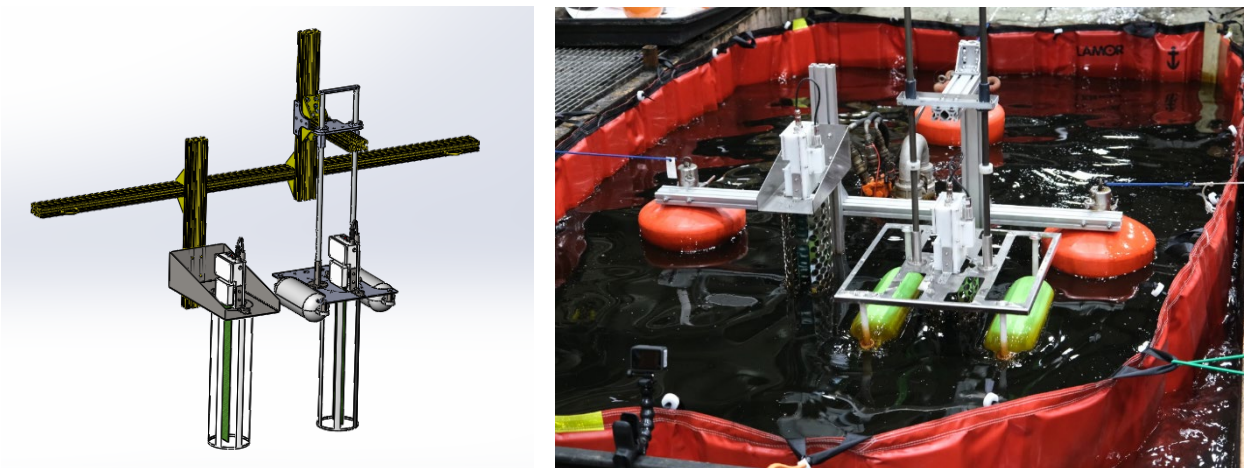
Figure 2.91: Left: Skimmer bridge. Right: Skimmer mount fully assembled.
