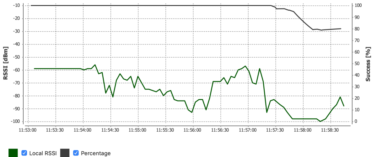
Figure 2.63: Xbee Pro S1 range test results
