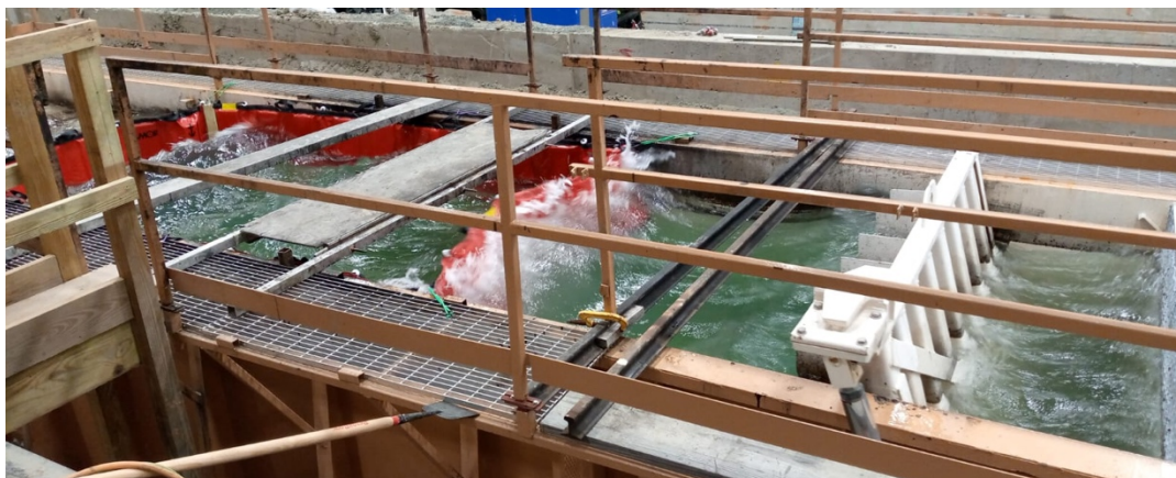
Figure 4.2: Wave tank used for dynamic tests.
