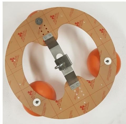
Figure 2.78: Floating configuration for the handheld sensor
