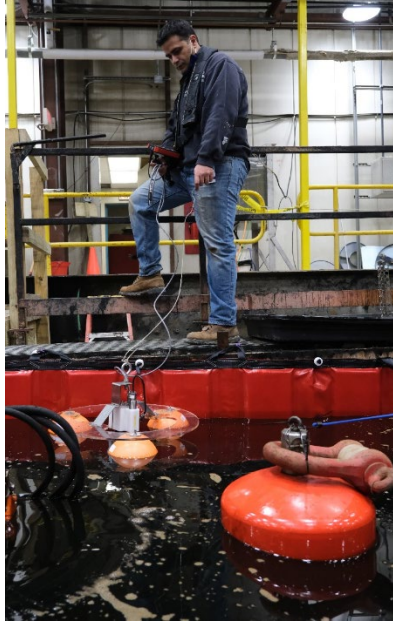
Figure 4.8: Handheld sensor on bouy in wave tank.
