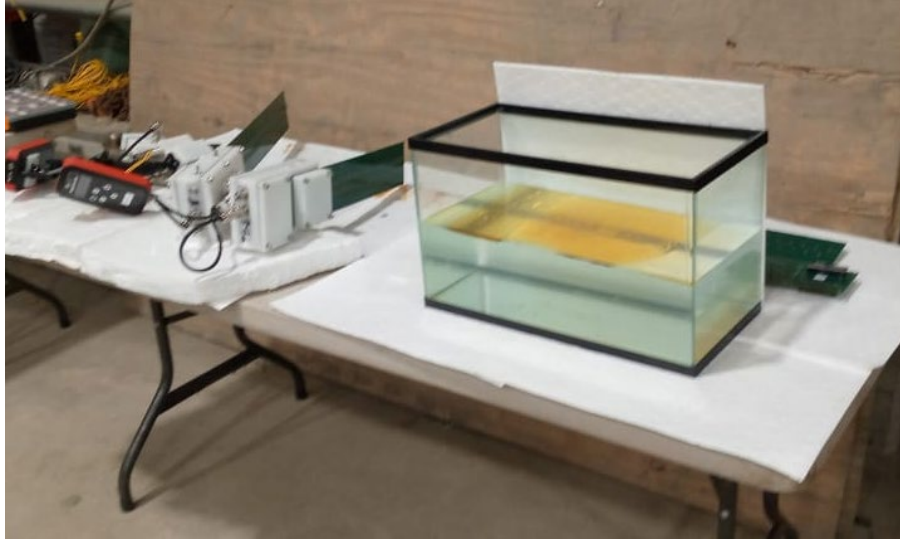
Figure 4.1: Glass fish tank used for static tests.
