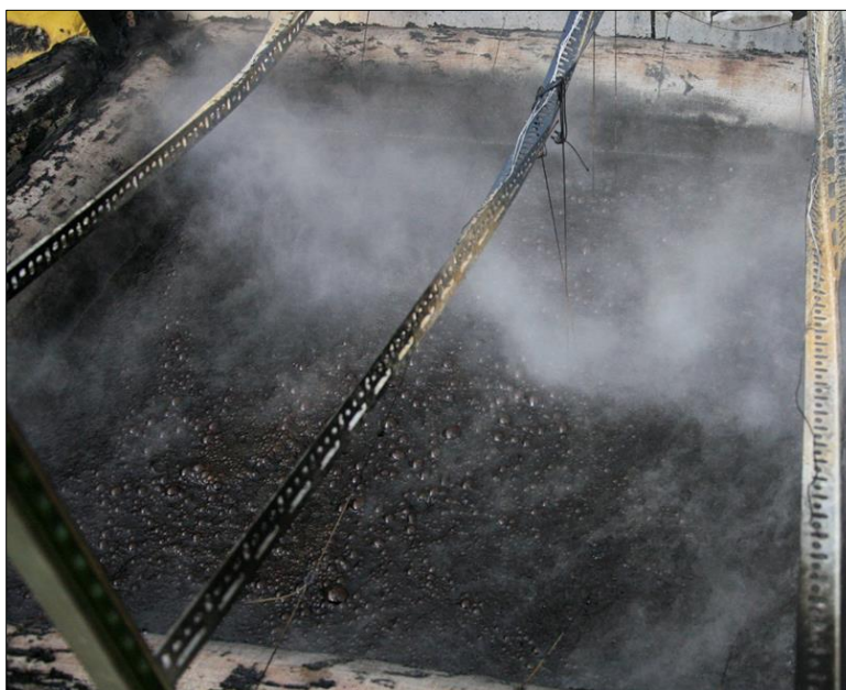
Figure 149 - Foaming then extinction – Baseline (HOOPS crude oil; Pool dimensions: 1.7 m by 1.9 m)
