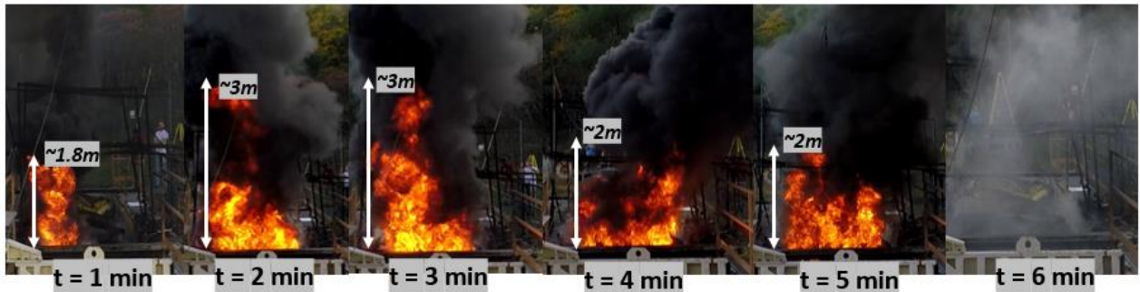
Figure 75 - Flame behavior for baseline case – No wave with bunker fuel
