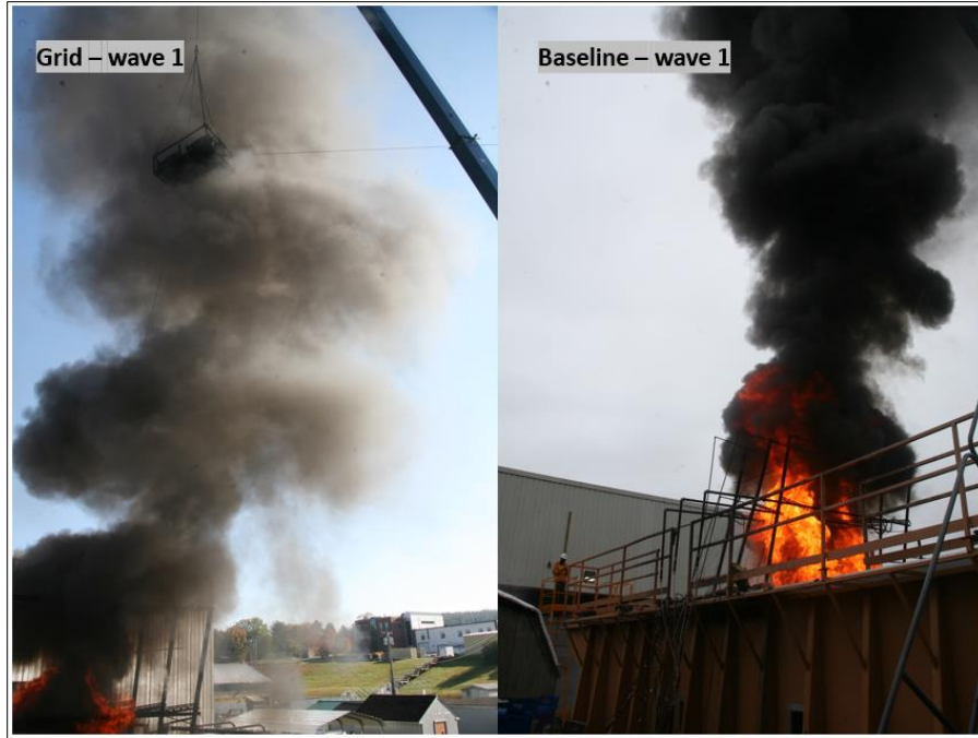
Figure 83 - Smoke visualization of grid FR and baseline case with wave 1
