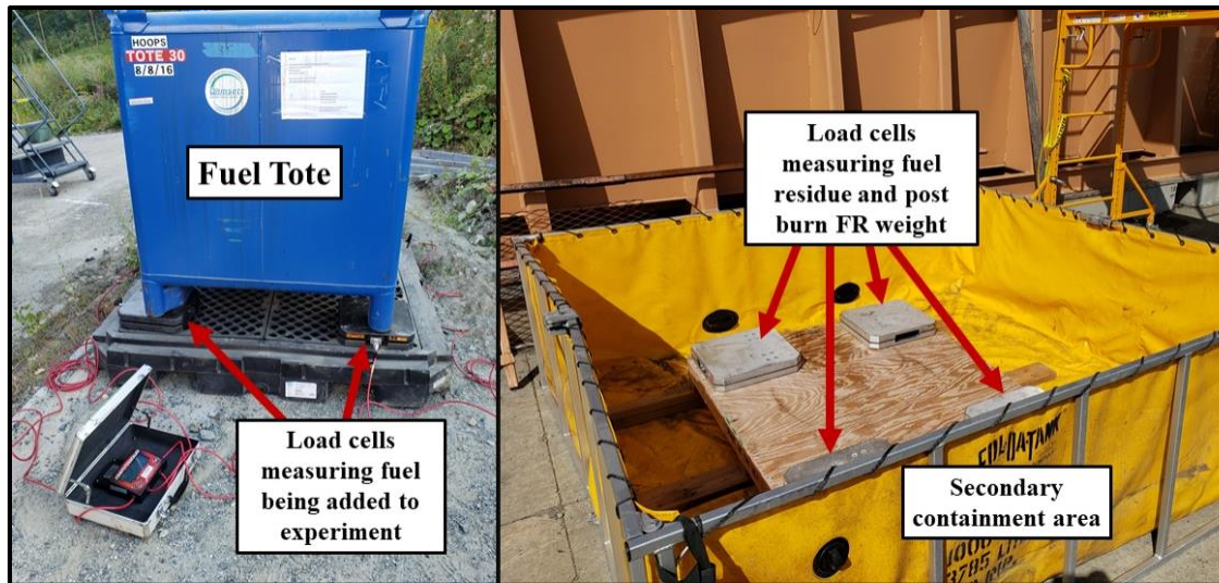
Figure 47 - (left) Fuel tote placed on load cells to measure the amount of fuel added to each experiment. (right) Load cells in a secondary containment area to measure fuel residue on FR's
