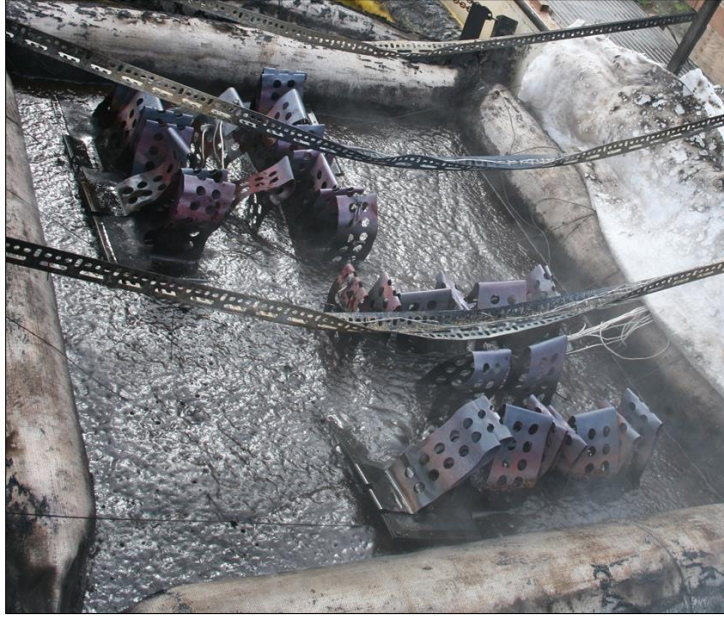
Figure 150 - Foaming then extinction – Ruffled metal FR (HOOPS crude oil)
