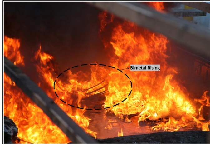
Figure 80 - Bimetal FRs raising with high temperatures – Wave 1 with HOOPS crude Oil
