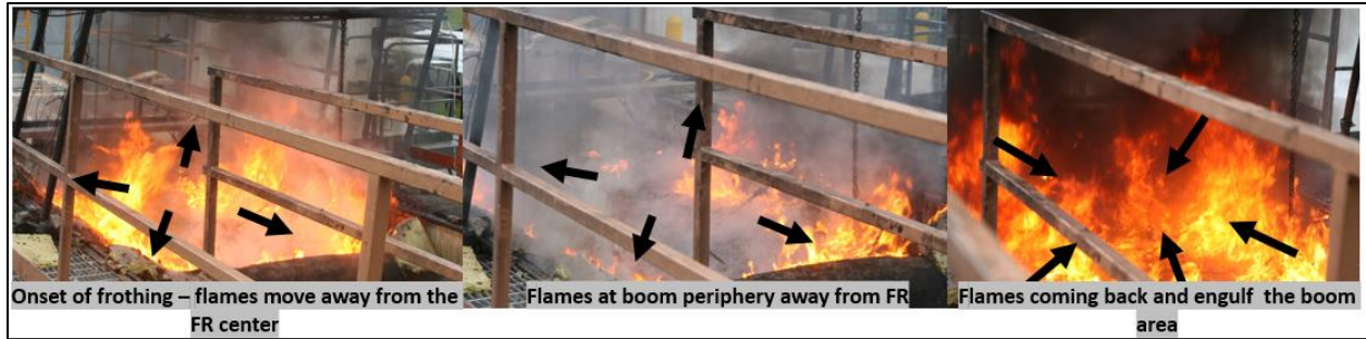
Figure 111 - Foaming cycle observed in Phase II experiments at CRREL with bimetal FR in wave 1 condition with Hoops crude oil
