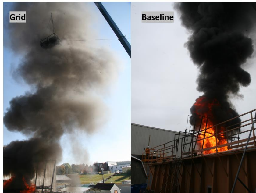
Figure 5 - Phase II – Smoke visualization of grid FR and baseline case with wave 1
