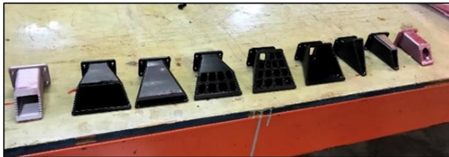
Figure 7: Suction Nozzle Test Setup (Nozzles 1-9 from left to right)
