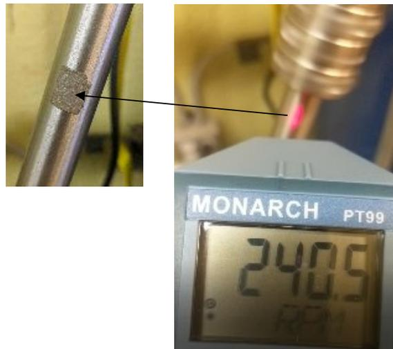
**Figure 22: Digital readout of shaft speed.**
