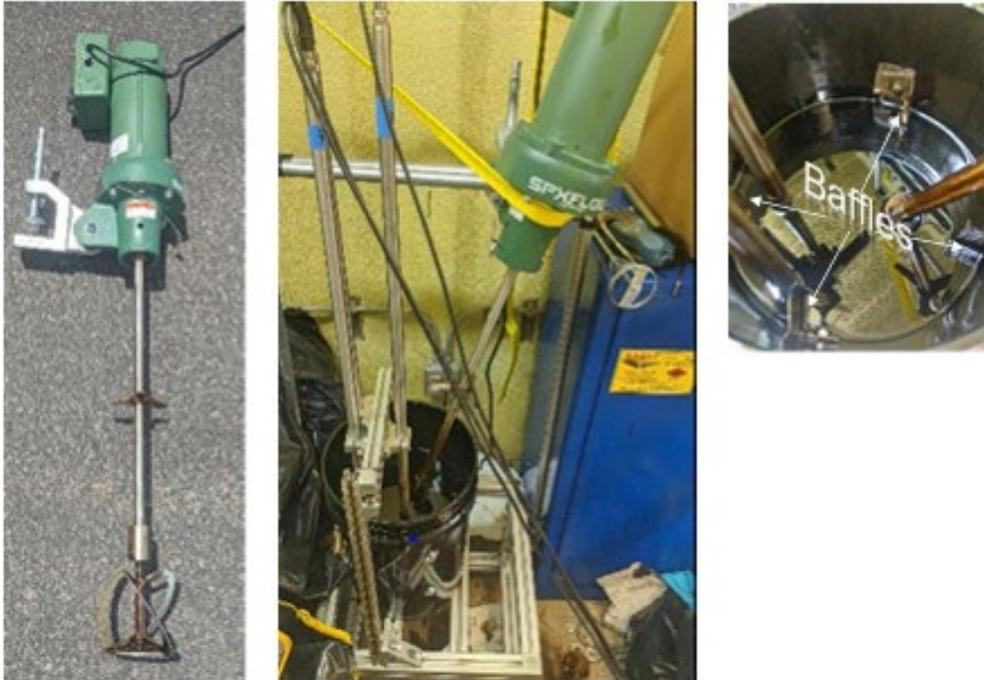
**Figure 21. Emulsion Mixing Apparatus and Motor Shaft**
