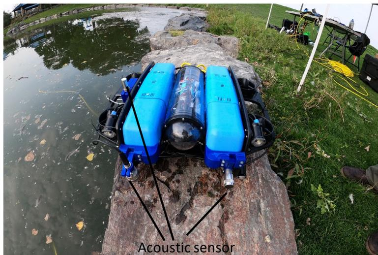
**Figure 16: BlueROV2 with acoustic sensors.**
