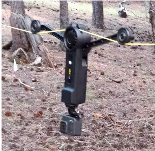
**Figure 9: Wiral Cable Cam and GoPro.**
