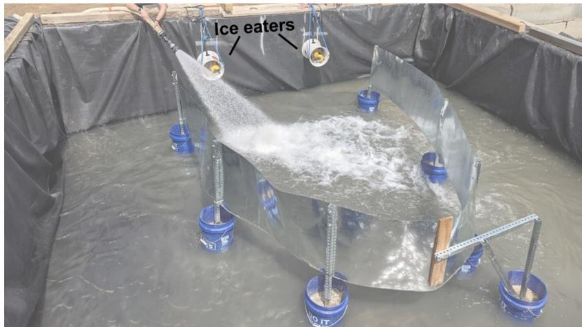
**Figure 47. Finished tank with sand layer and pond liner.**
