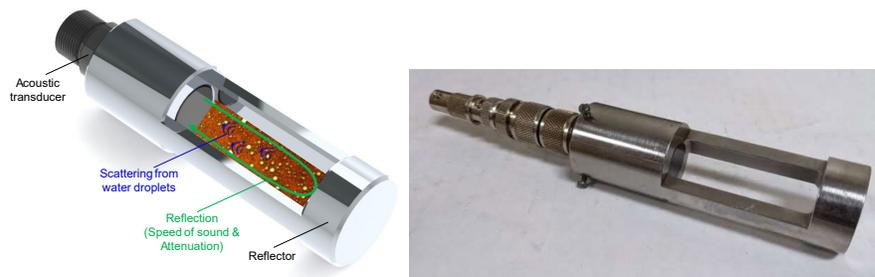
**Figure 27. Transducer with reflector as drawn (left), as fabricated (right).**
