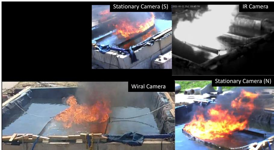
**Figure 53.** Images of the burning HOOPS from moving and stationary visible light cameras as well as an IR camera.
