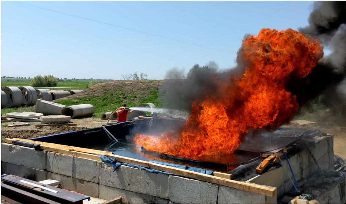
**Figure 8. ISB of 19 Liters (5 gallons) of HOOPS in a simulated boom.**
