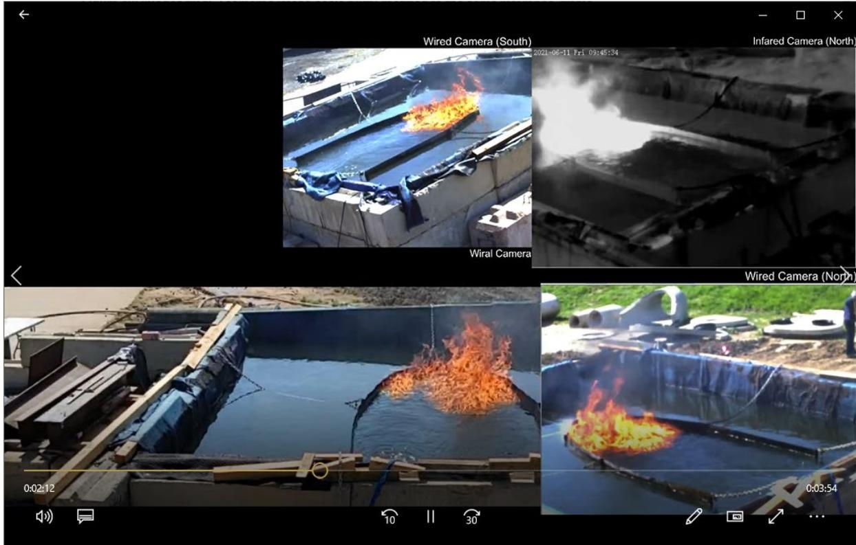
**Figure 5: The meso-scale saved video, which looks exactly like the computer display and is configurable.**
