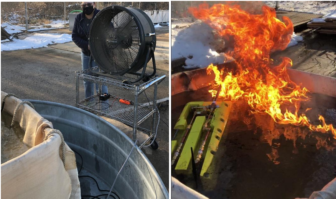
Figure 15: Dodecane Wind Burn at Phoenix Facility
