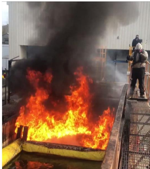
Figure 22: Frazil Ice Weathered HOOPS Burn at CRREL
