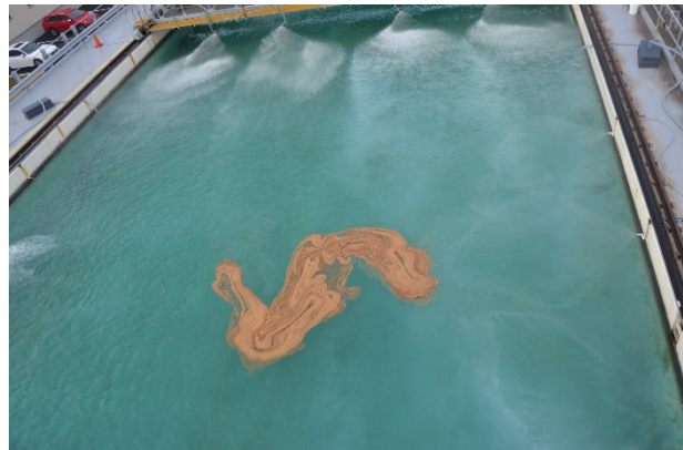
Figure 4: Redesigned side spray barriers, showing i) schematic layout, ii) manifold, iii) individual spray nozzle, and iv) containing a small slick of oil.
