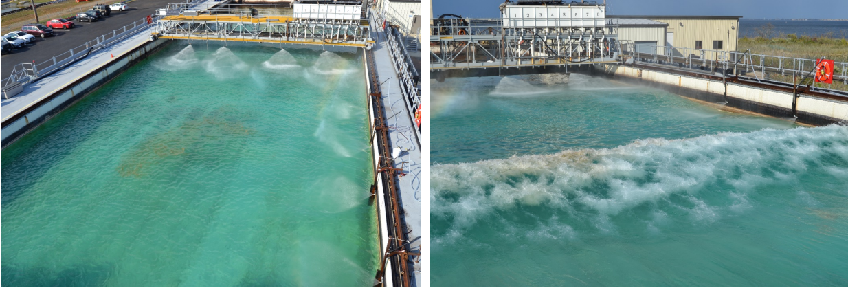
Figure 3: Prototype side sprayers tested with waves.
