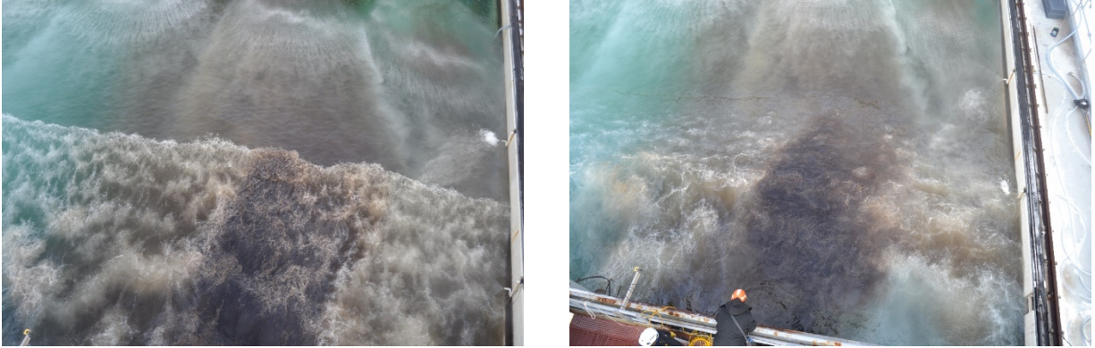
Figure 15: Breaking Wave 2 impacting treated test slick.
