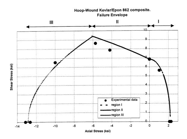
Figure 11. Multiaxial Failure Strength Envelope for Kevlar/Epoxy Composite
