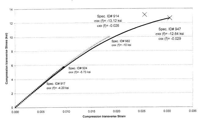
Figure 9. Transverse Compressive Stress-Strain Behavior of Hoop-Wound Kevlar/Epoxy Composite
