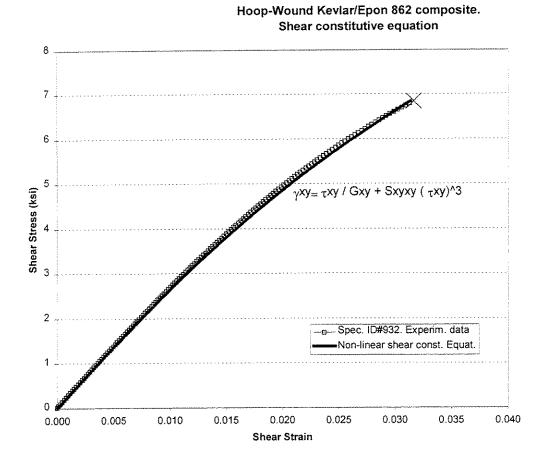
Figure 10. Nonlinear Shear Constitutive Equation for Hoop-Wound Kevlar/Epoxy Composite
