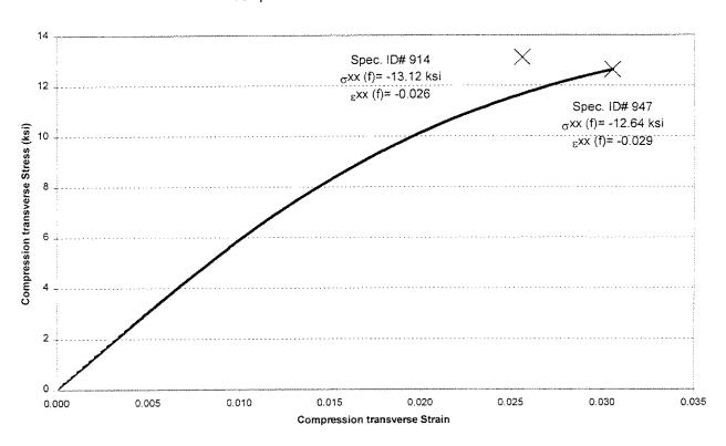
Figure 5. Transverse Compressive Stress-Strain Behavior of Hoop-Wound Kevlar/Epoxy Composite
