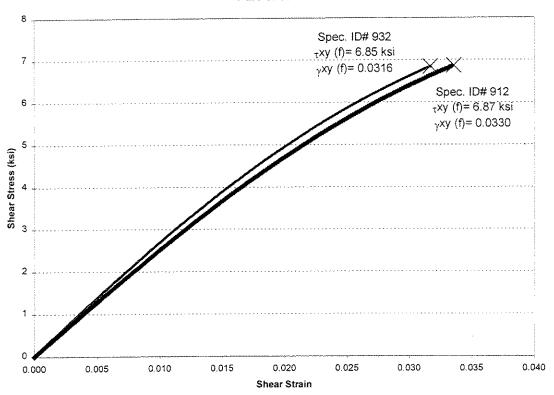
Figure 6. Pure shear stress-strain behavior of hoop-wound Kevlar/epoxy composite
