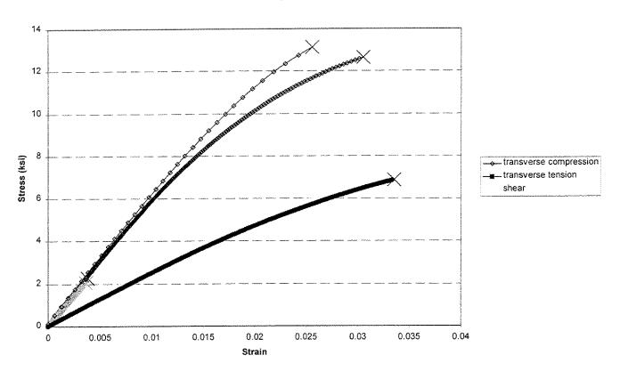
Figure 7. Transverse Axial and Pure Shear Stress-Strain Behavior of Hoop-Wound Kevlar/Epoxy Composite
