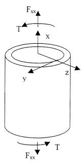
Note that all the results are shown in the structural coordinates [x, y, z], where x represents the transverse direction of fibers, and y, the longitudinal direction of fibers.
