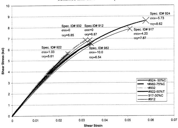
Figure 8. Multiaxial Mechanical Behavior of Kevlar/Epoxy Subject to Combined Transverse Axial and Pure Shear Loading
