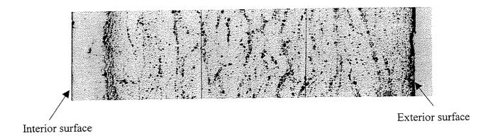
Figure 2. Microstructure of the Kevlar/Epoxy Composite
