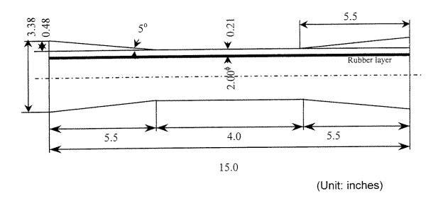
Figure 1. Kevlar/Epoxy Composite Test Specimen Geometry
