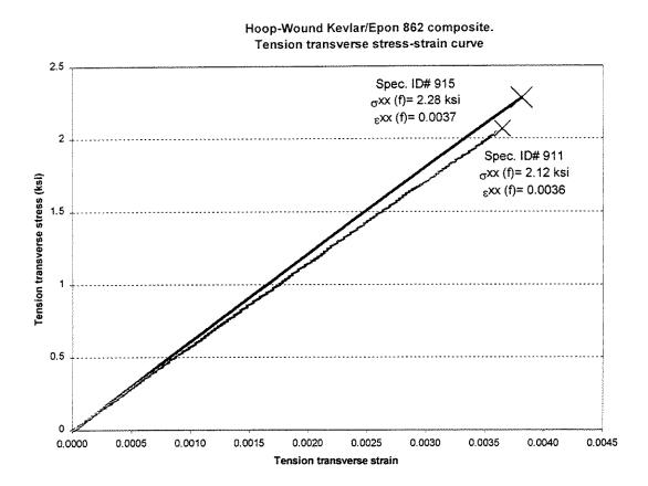
Figure 4. Tensile Transverse Stress-Strain Behavior of Hoop-Wound Kevlar/Epoxy Composite
