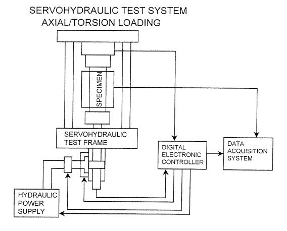
Figure 3. Servo-Hydraulic Multiaxial Material Test System
