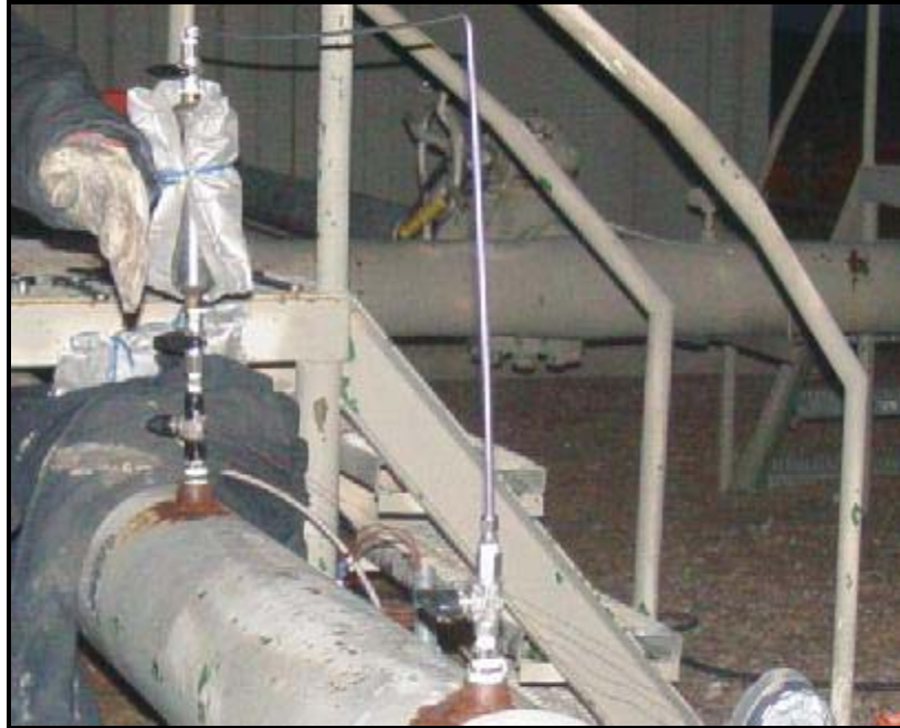
Figure 10. Configuration of the equipment used for collecting samples with the Pitot and Bypass method at the Powder Wash field site.
