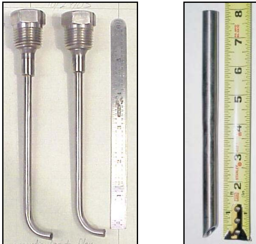
Figure 11. Sampling probes used for the Powder Wash tests. Left, curved probes for the Pitot and Bypass method; right, example of a straight probe used for the other sampling methods.
