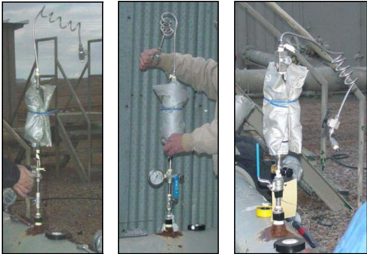
Figure 9. Configuration of the equipment used for collecting samples at the Powder Wash field site. Left, Controlled Rate Purge; center, Fill-and-Empty; right, High-Pressure Helium Displacement.
