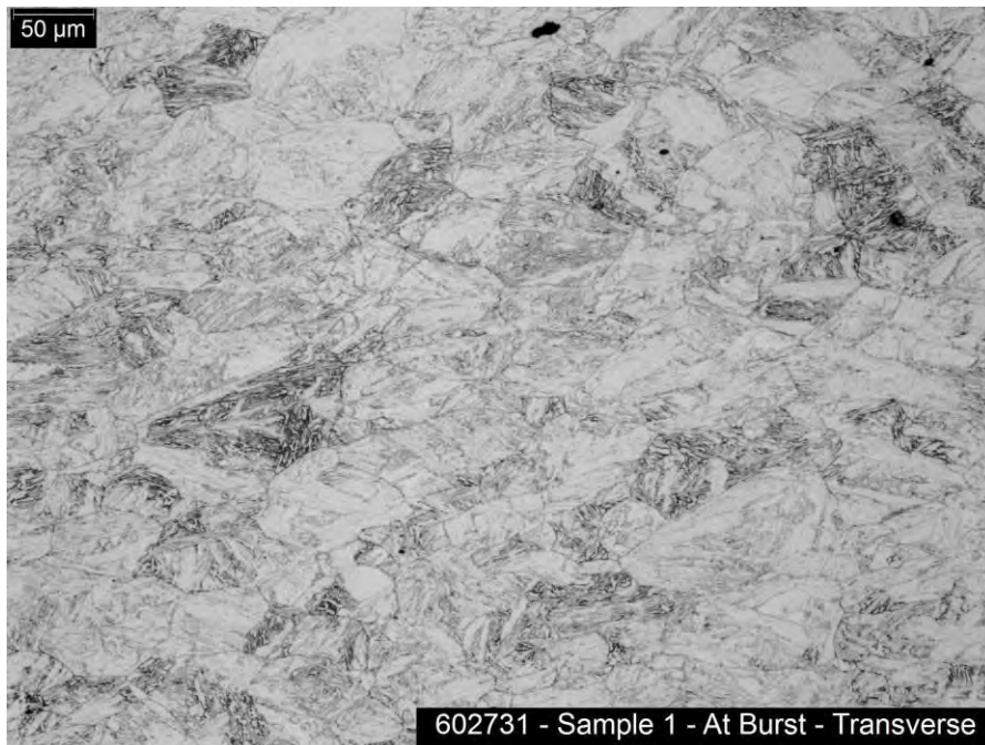
Figure 22: Sample 1 – Micro photograph of Transverse cross-section at Burst, Grain Size No. 7
