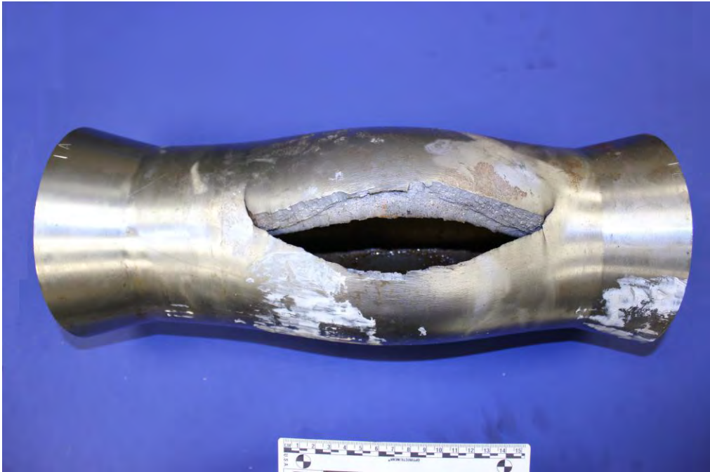
Figure 3: As Received Photograph – Sample 2 – Top View of Base Case at Burst (scale in mm)
