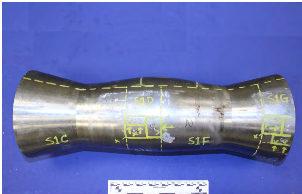
Figure 7: Layout Photograph – Sample 1 - Bottom View of Reduced Case, 180° from Burst (scale in mm)
