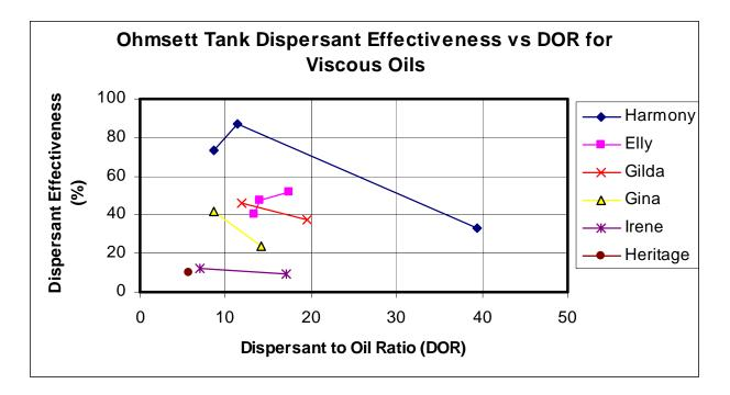
Figure 4. Ohmsett Test Tank Results: Dispersant Effectiveness versus DOR by Oil Name
