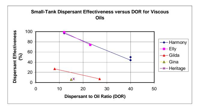
Figure 2. Small-Scale Tank Test Dispersant Effectiveness versus DOR by Oil Name
