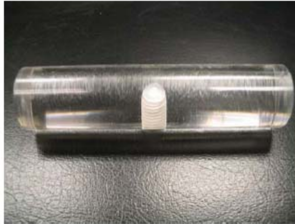
Figure 4. Acrylic tip for the T-bar (from Vanka, 2004)
