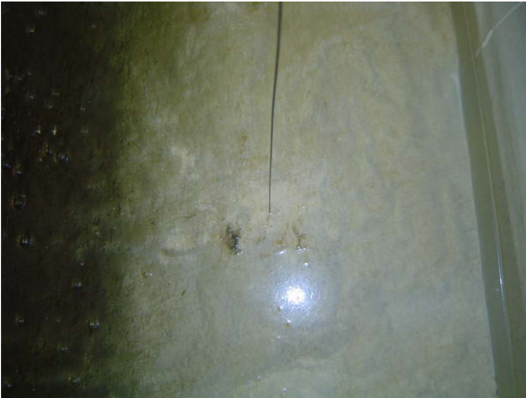
Figure 7. Slight disturbance in soil surface after deployment
